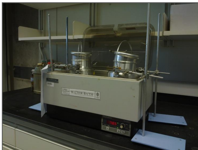
Figure 3.2-Preparation of Samples in Water Bath
