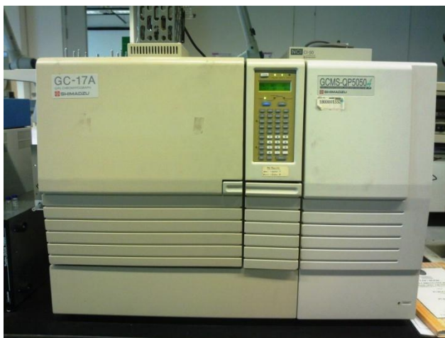
Figure 3.3-Shimadzu 5050 GC Coupled with Shimadzu 5973 with Mass Selective Detector
