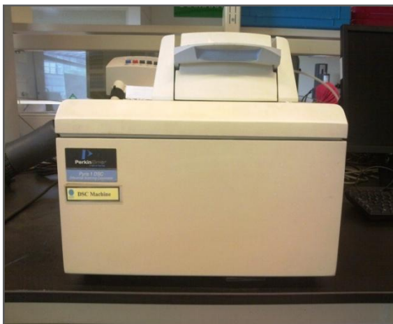
Figure 3.5-Differential Scanning Calorimetry (DSC)
