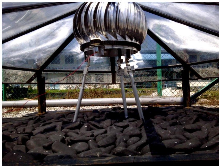
Figure 4.2.7: Turbogenerator Prototype (Front view: With Tripod stand)
