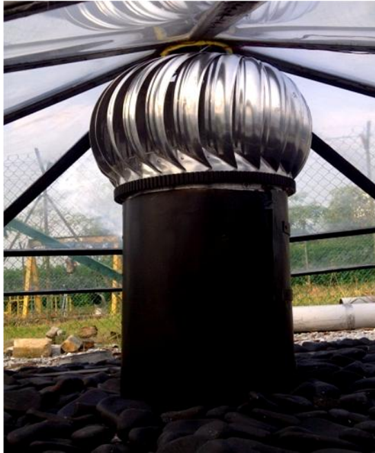
Figure 4.2.8: Turbine with cylindrical enclosure for Case 3
