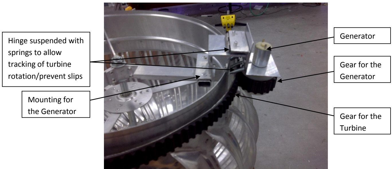
Figure 4.2.5: Flexible Turbogenerator coupling (Bottom view)
