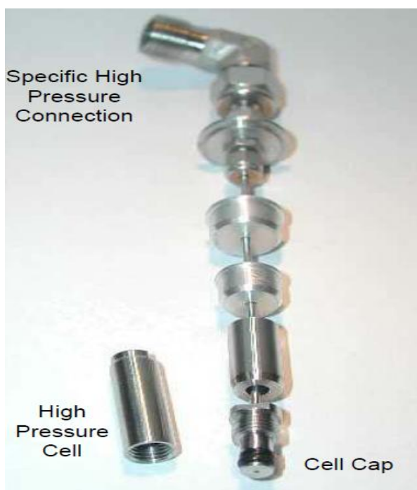
Figure 14 - Specific high-pressure vessel
