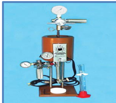
Figure 20: HPTP press filter
