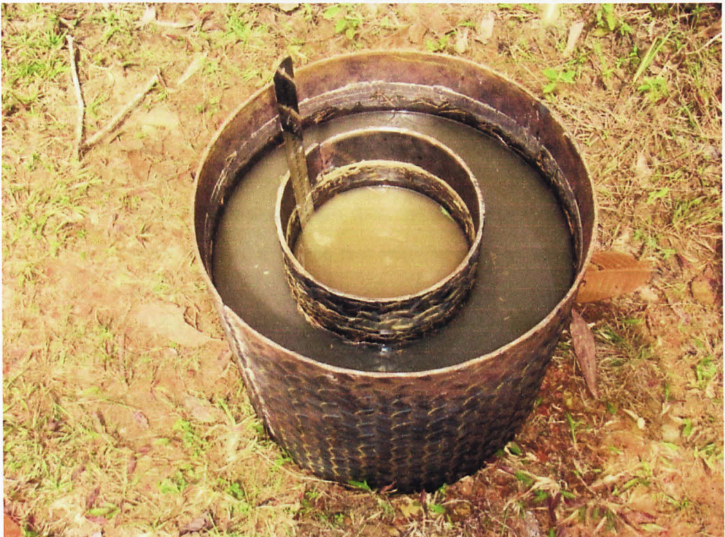
Figure 3.5: Double Ring Infiltrometer test
