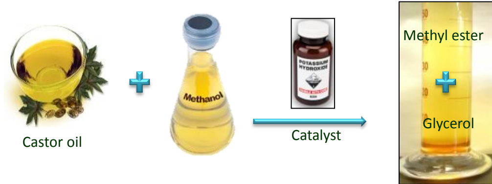
Figure 10: Overall transesterification reaction of castor oil
