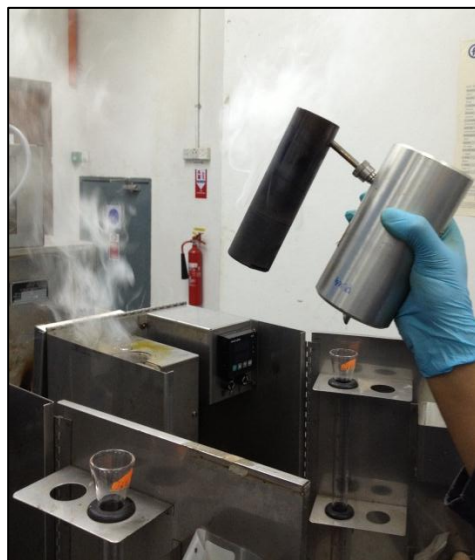
Figure 22: Retort was leaking due to plugging of base fluid
