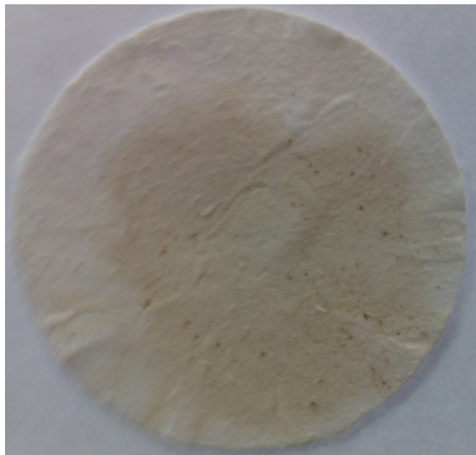
Figure 16 : Asphaltene precipitates on glass fiber filter paper
