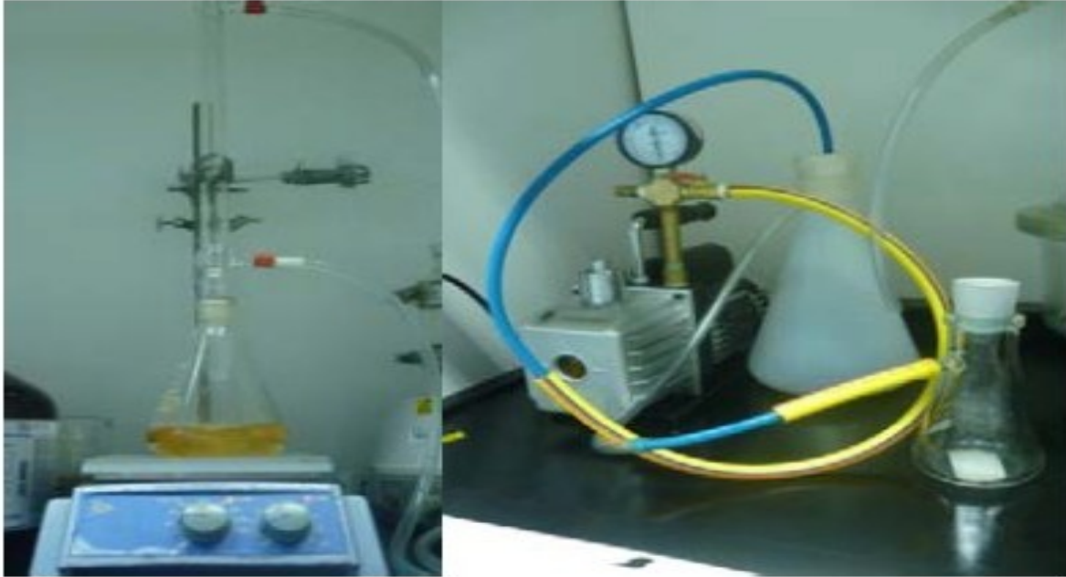
Figure 6 : Apparatus for ASTM D3279 -07 Standard Test Method for n-Heptane insoluble
