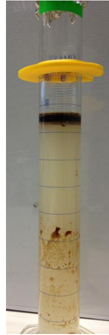
Figure 19: Effluent from alkaline flooding (0.5% NaOH)
