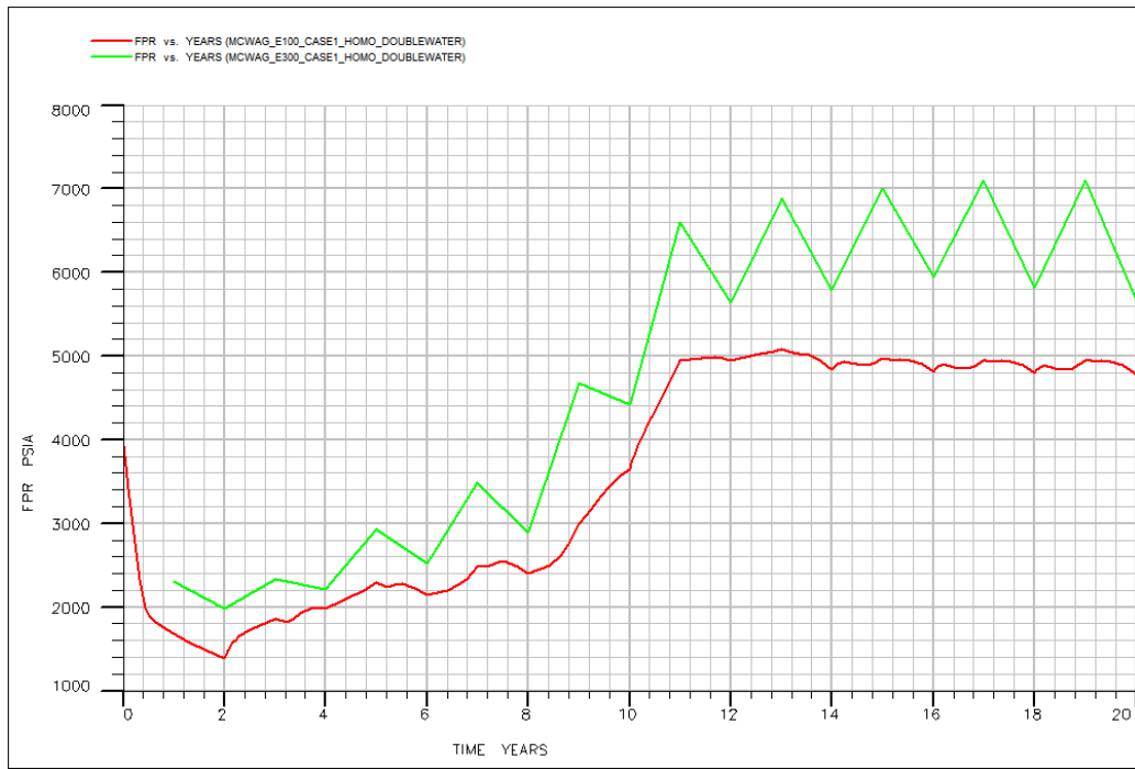
Figure 25: Reservoir Pressure for Double Water Injection Case
