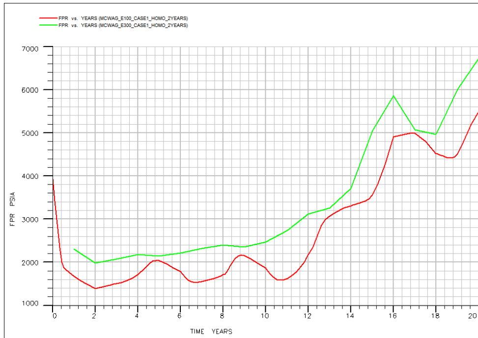
Figure 16: Reservoir Pressure for 2 Years WAG Cycle
