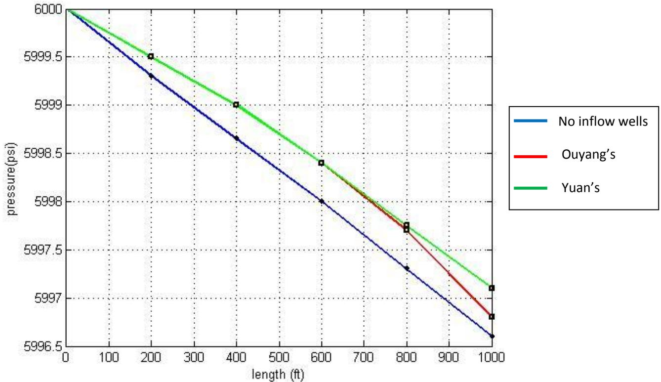
**Figure 4.3: Pressure analytical model for 6 in Tubing**
