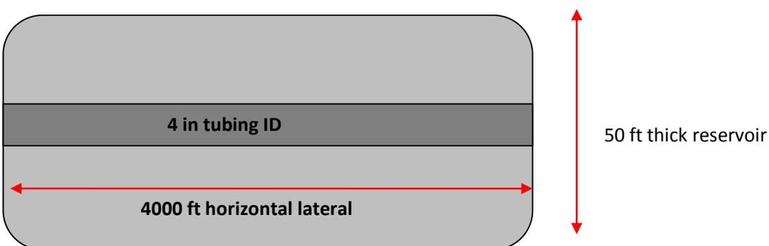
**Figure 4.4: Example of tubing setting in the formation**
