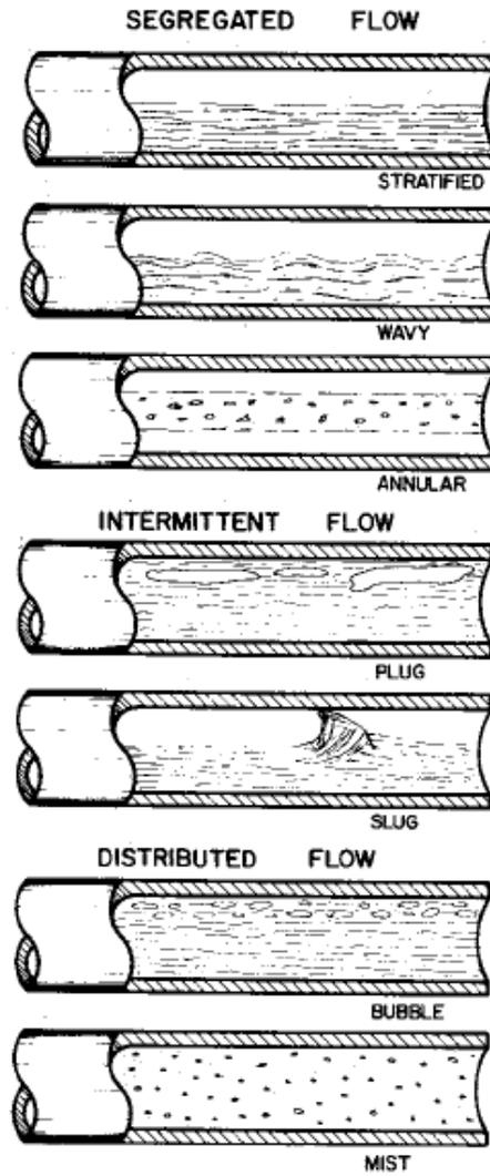
**Figure 2.1: Horizontal Flow Pattern**
