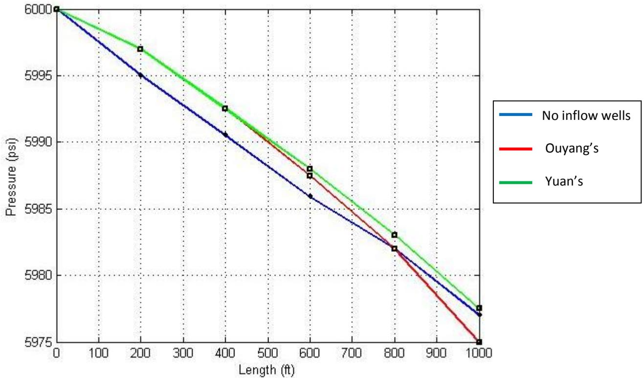
**Figure 4.1: Pressure drop analytical model for 4 in Tubing**
