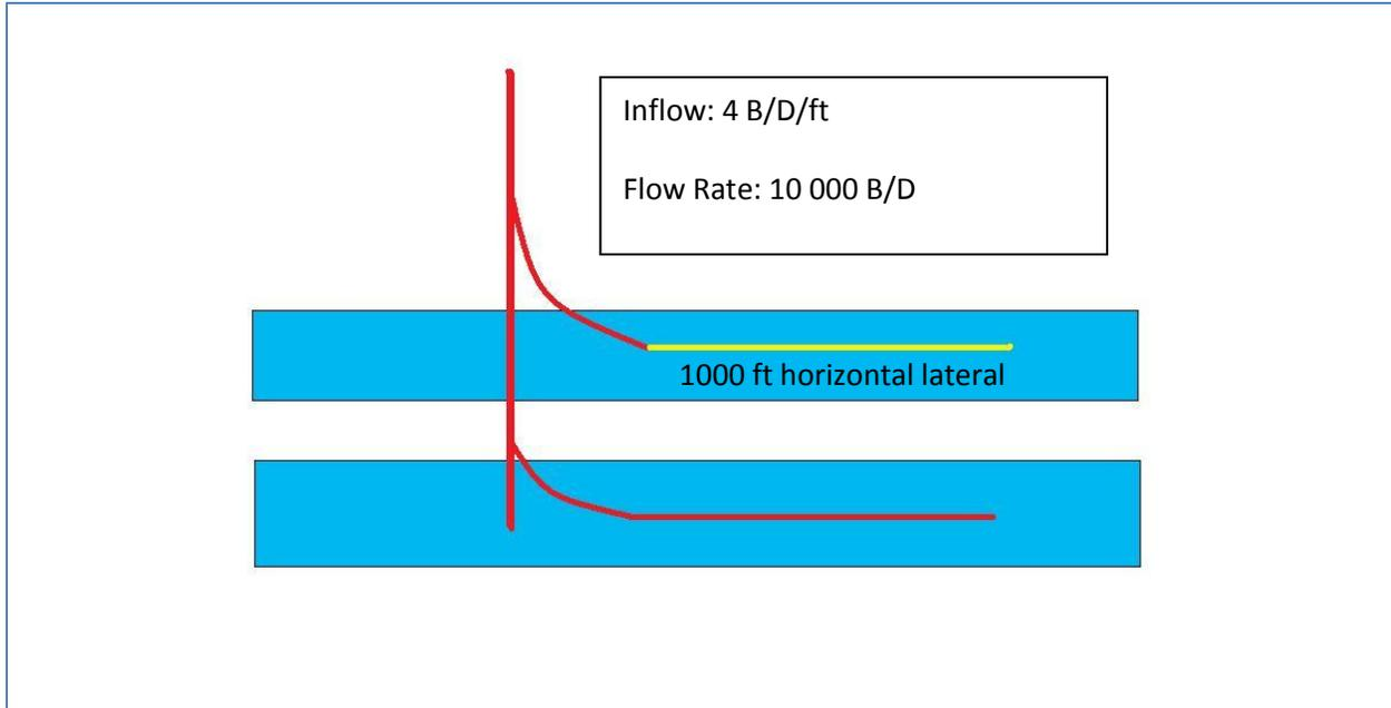
**Figure 3.2: Model assumption for horizontal lateral**
