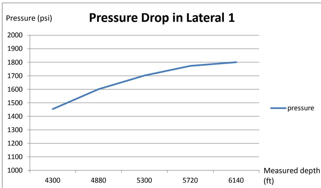
**Figure 4.5: Pressure drop analytical model in Lateral 1**
