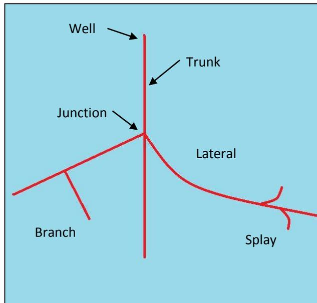
**Figure 1.1: Schematic diagram of a multilateral well**
