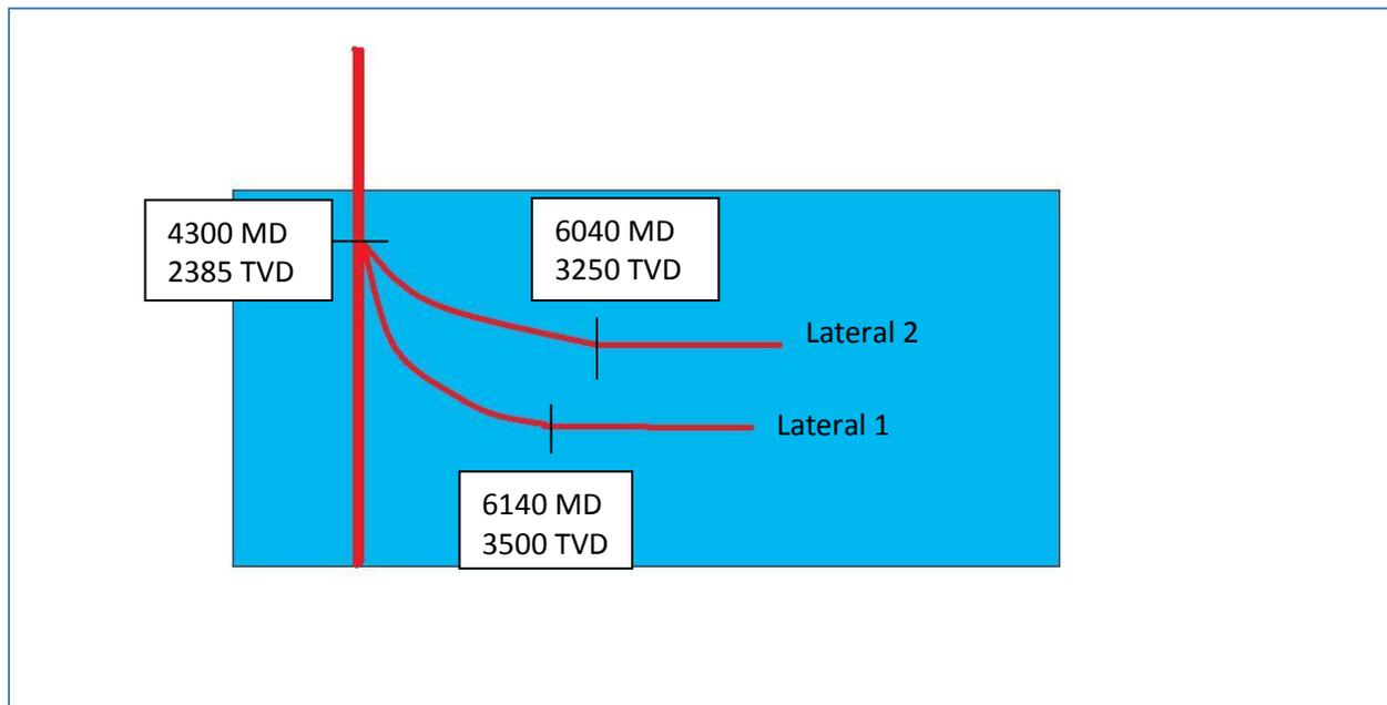
**Figure 3.3: Model Assumption for build-up lateral**
