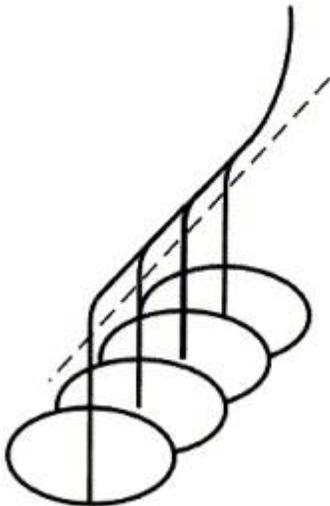
c) Multibranch well with fractured vertical branches (horizontal parent well is drilled above the reservoir).
