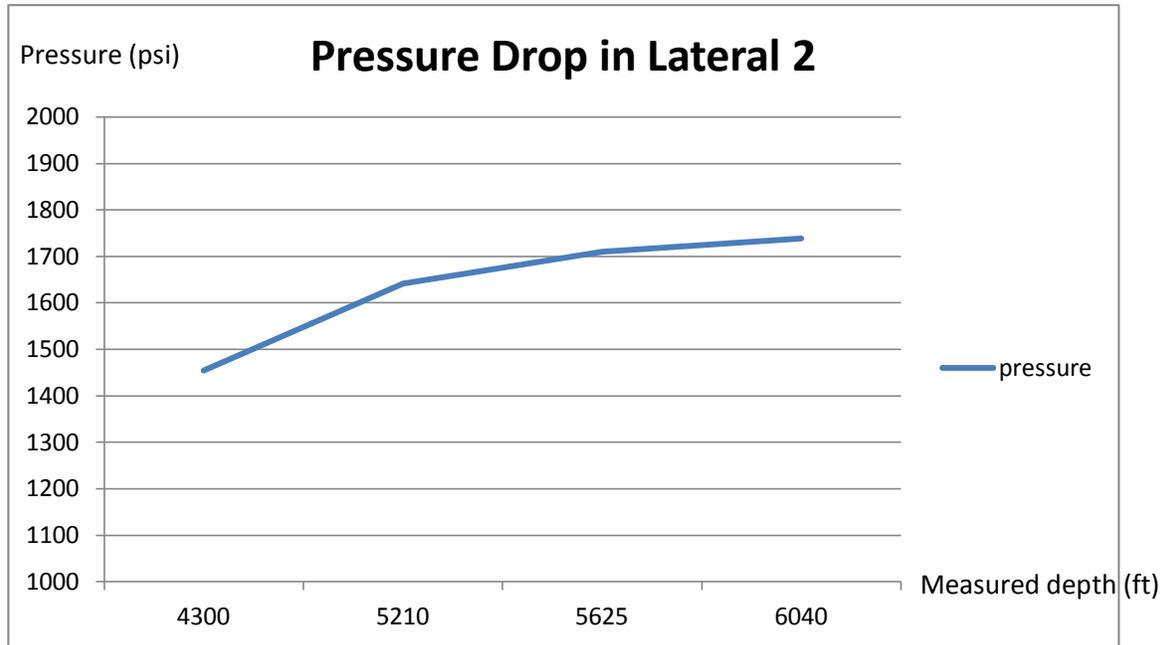
**Figure 4.6: Pressure drop analytical model in Lateral 2**
