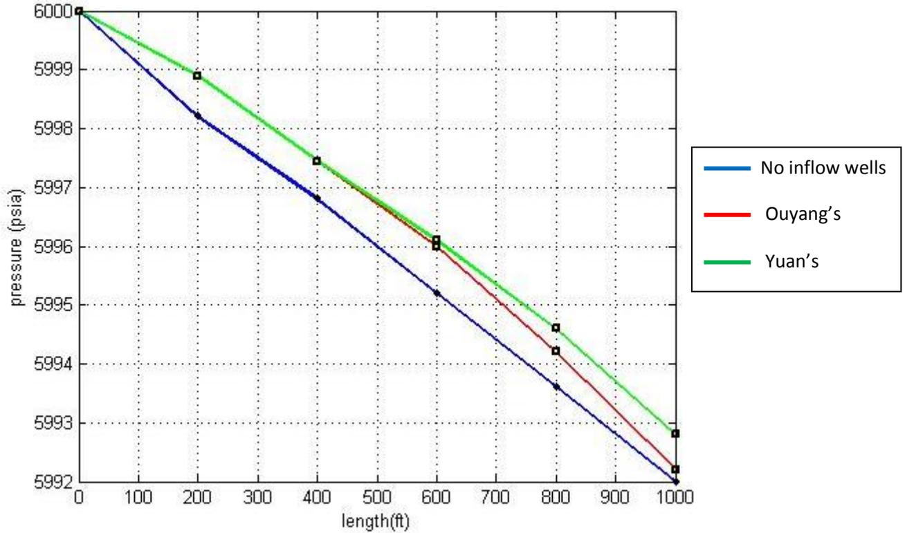
**Figure 4.2: Pressure drop analytical model for 5 in Tubing**
