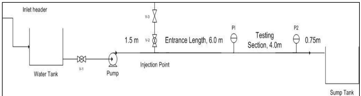
Figure 5: Project equipment setup
