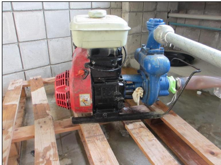
**Figure 15:** Engine pump
