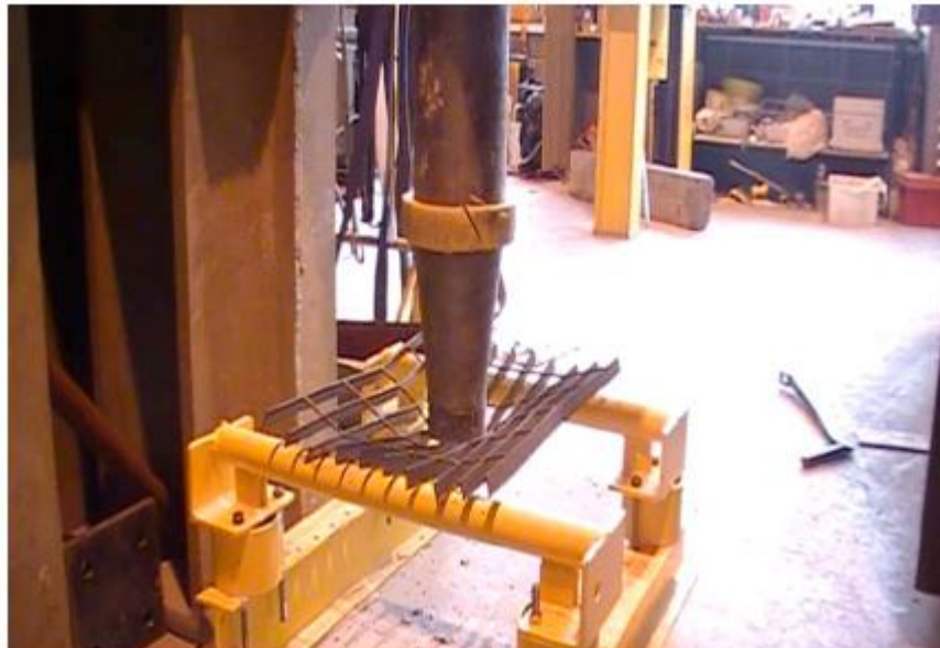
Figure 2.2 : Flowforge Open Grating after Impact from 76kg billet at 0.62m height
