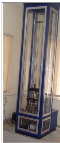
Figure 2.6: Falling weight impact test equipment
