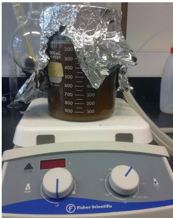
Figure 7.5: Raw Rice Husk treated with NaOH
