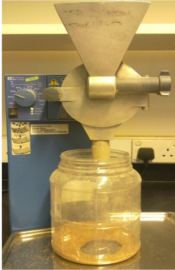
Figure 7.3: Grinder used for grinding process
