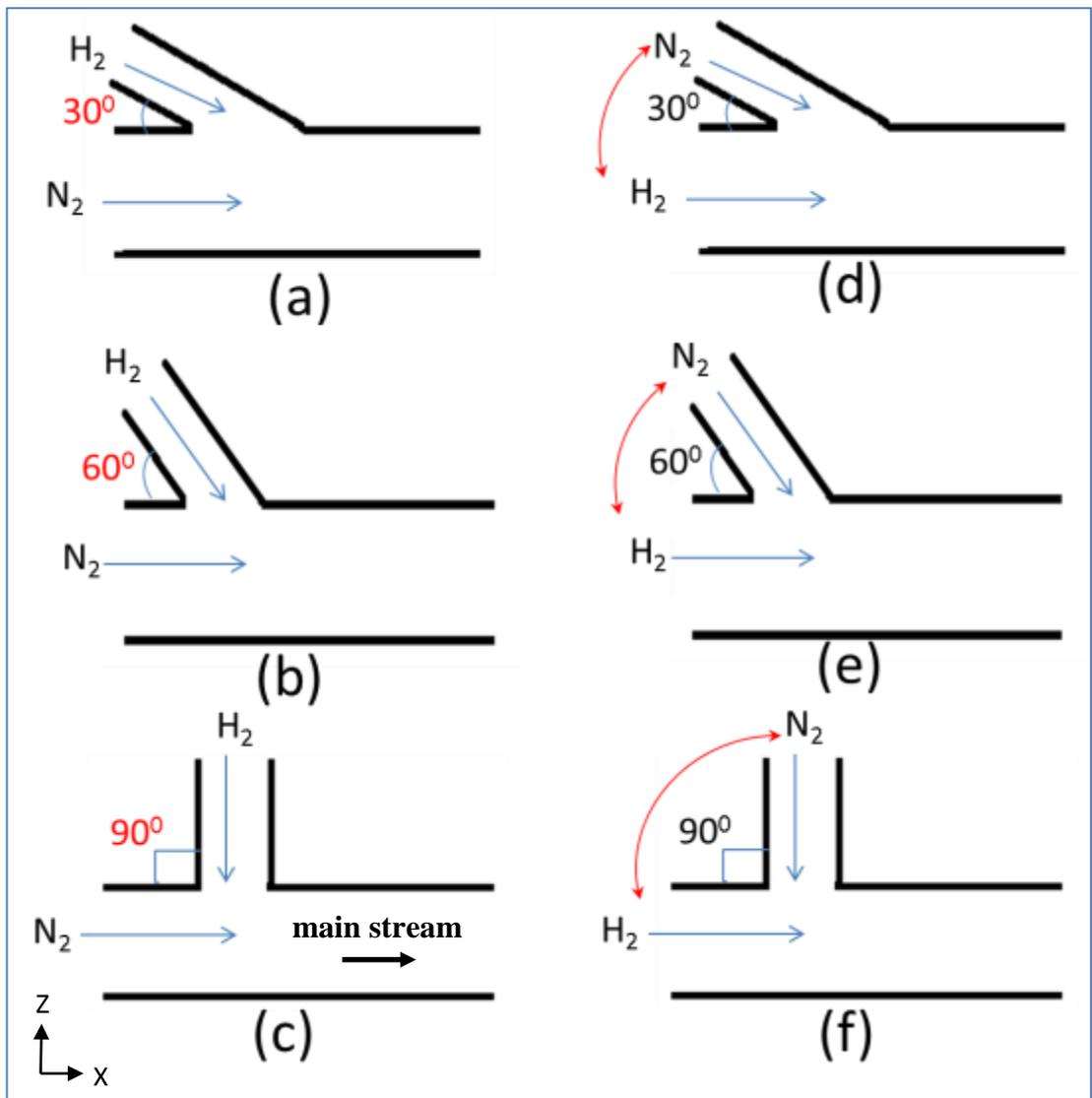
**FIGURE 3-3:** (a) Inlet geometry of  $30^\circ$  and nitrogen in the main stream, (b) Inlet geometry of  $30^\circ$  and hydrogen in the main stream, (c) Inlet geometry of  $60^\circ$  and nitrogen in the main stream, (d) Inlet geometry of  $60^\circ$  and hydrogen in the main stream, (e) Inlet geometry of  $90^\circ$  and nitrogen in the main stream, (f) Inlet geometry of  $90^\circ$  and hydrogen in the main stream.
