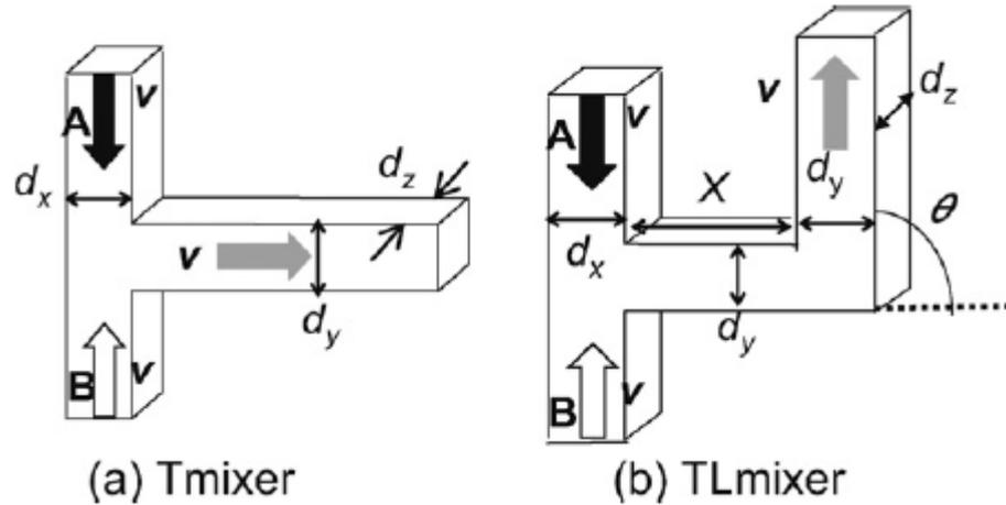
**FIGURE 2-5:** Schematic of T-mixer and TL-mixer (N. Aoki, 2010)
