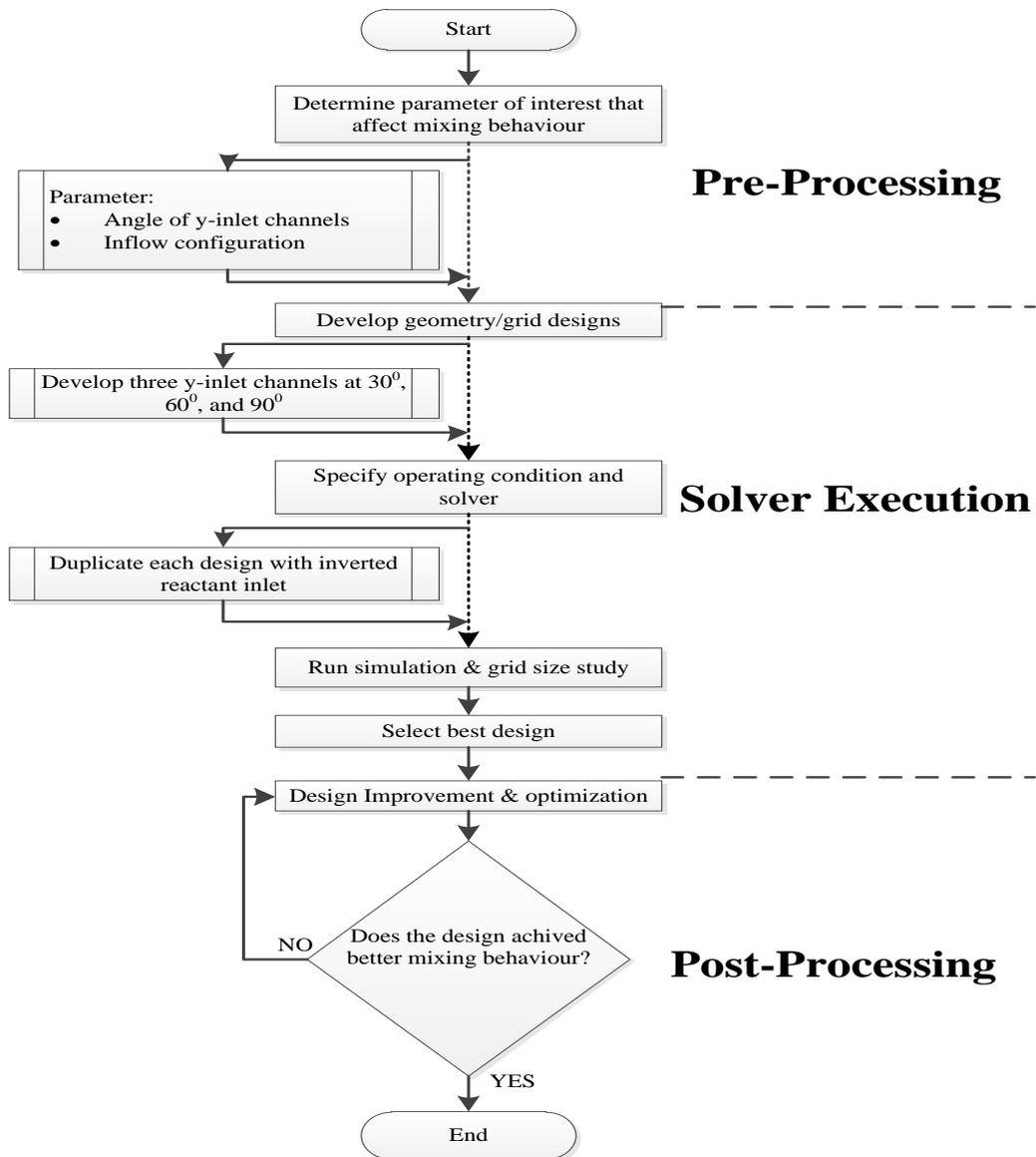
FIGURE 3-1: Block Diagram for Simulation Flow
