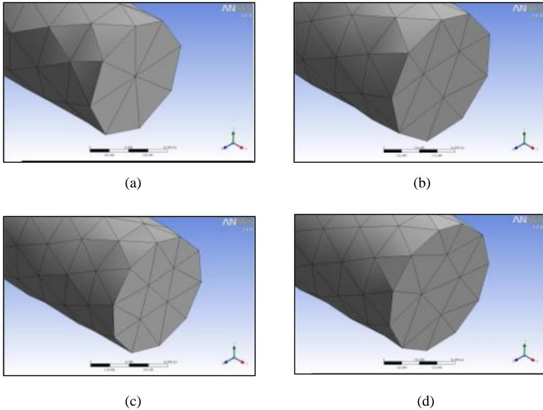
**FIGURE 4-1:** Meshing (a) 250,000 nodes (b) 330,000 nodes (c) 410,000 nodes (d) 510,000 nodes
