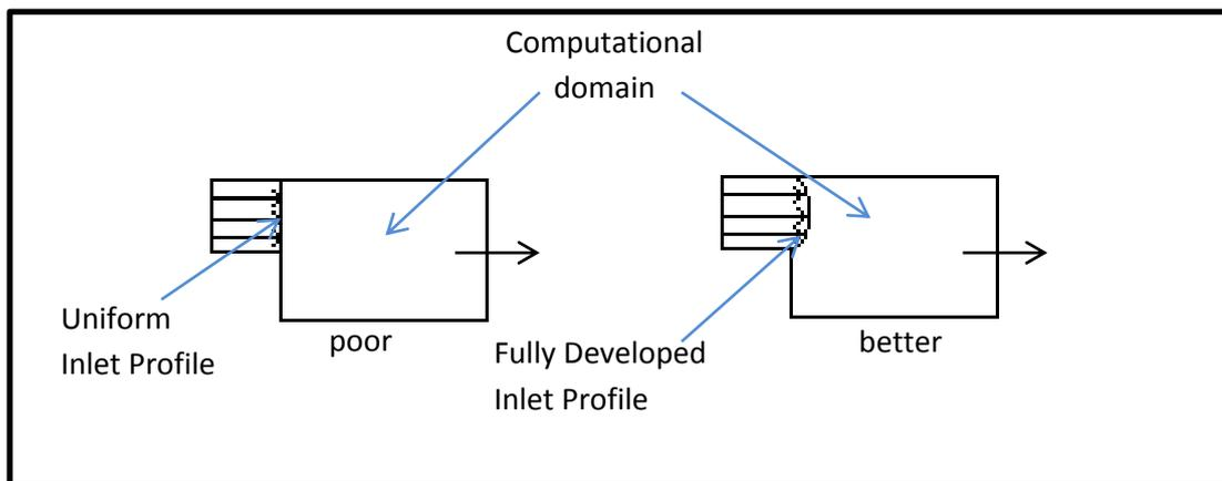
**FIGURE 2-2:** Velocity Profile Comparison
