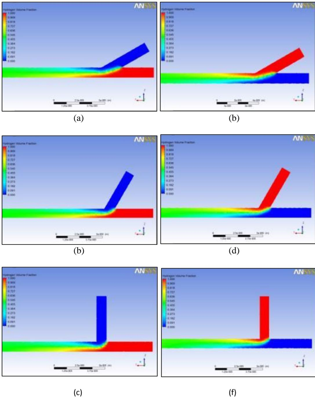
**FIGURE 4-4:** Hydrogen fraction contour (a) Inlet geometry of  $30^\circ$  and hydrogen in the main stream, (b) Inlet geometry of  $30^\circ$  and nitrogen in the main stream, (c) Inlet geometry of  $60^\circ$  and hydrogen in the main stream, (d) Inlet geometry of  $60^\circ$  and nitrogen in the main stream, (e) Inlet geometry of  $90^\circ$  and hydrogen in the main stream, (f) Inlet geometry of  $90^\circ$  and nitrogen in the main stream
