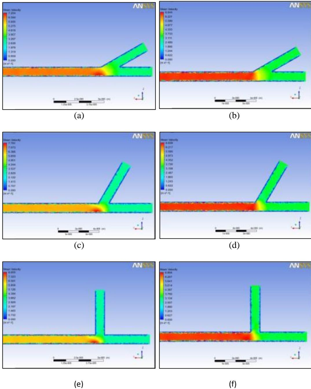
**FIGURE 4-3:** Velocity contour plot: (a) Inlet geometry of 30° and hydrogen in the main stream, (b) Inlet geometry of 30° and nitrogen in the main stream, (c) Inlet geometry of 60° and hydrogen in the main stream, (d) Inlet geometry of 60° and nitrogen in the main stream, (e) Inlet geometry of 90° and hydrogen in the main stream, (f) Inlet geometry of 90° and nitrogen in the main stream
