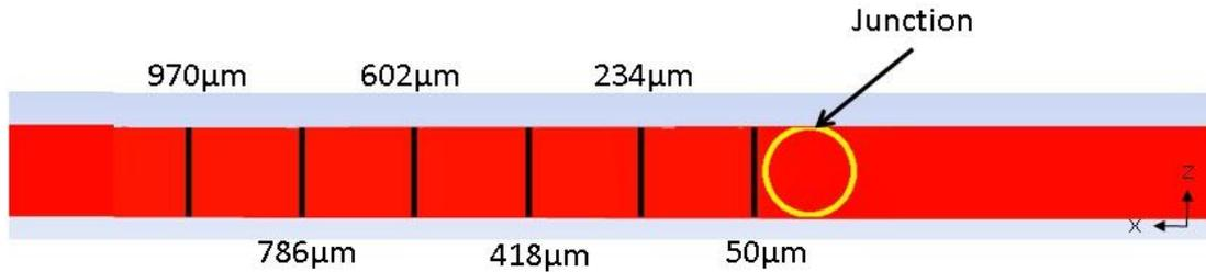
**FIGURE 4-6:** Position of hydrogen volume fraction profile taken along X-axis
