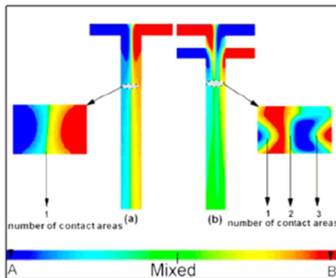
**FIGURE 2-4:** Mass fraction contour in T- and DT-micromixer
