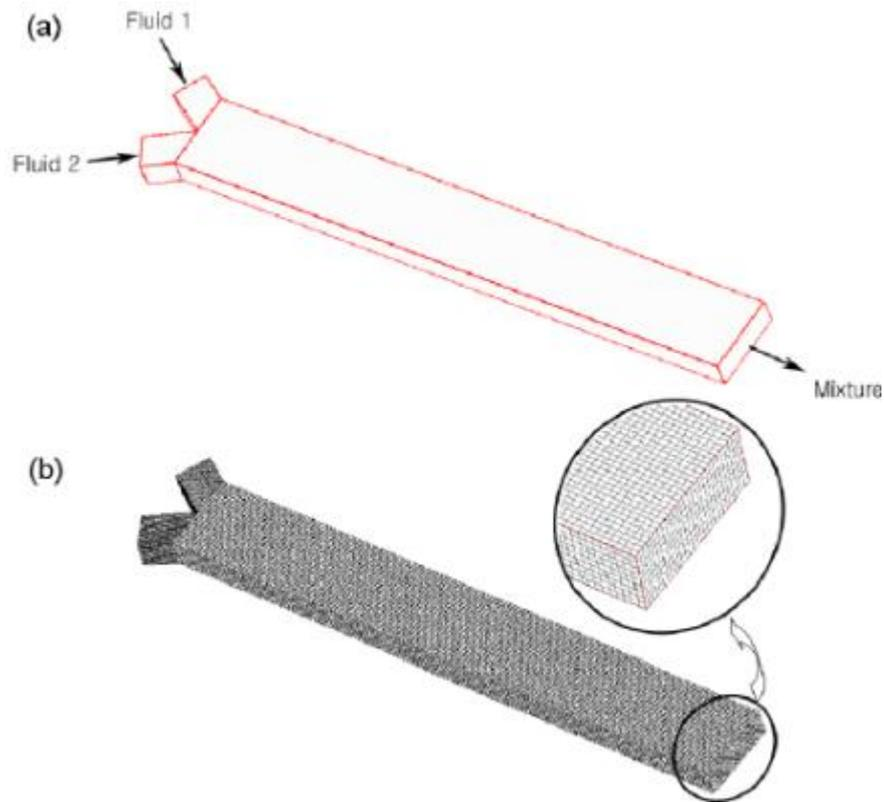
**FIGURE 2-1:** Y-shaped microchannel and generated grid (Maeng, Yoo, & Song, 2006)
