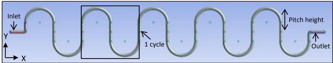
**FIGURE 3-2:** General microreactor geometry (Rosli, 2012)
