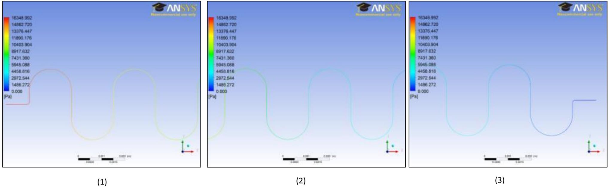
FIGURE C-1: Pressure contour for 30<sup>0</sup> angle and hydrogen in main stream
