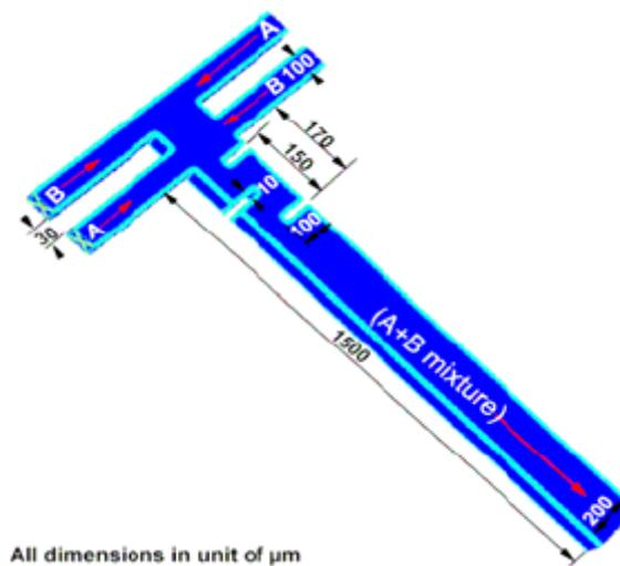
**FIGURE 2-3:** Passive DT-micromixer(Elmabruk A. Mansur, 2008)
