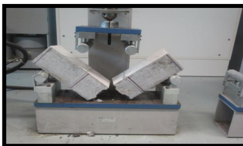
Figure 4.1 : beam with no fiber addition
