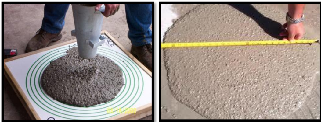
Figure 3.7: Slump flow and slump T_{50} test
