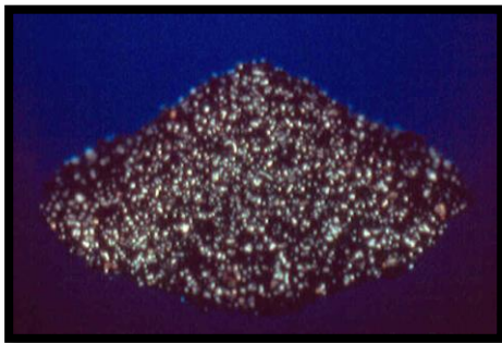
Figure 2.7 : Bulk Fly Ash
