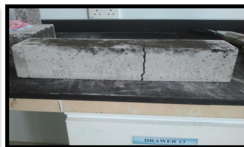
Figure 4.2 : beam with fiber addition
