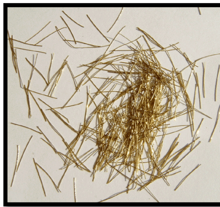
Figure 3.2 : Steel fiber - straight type
