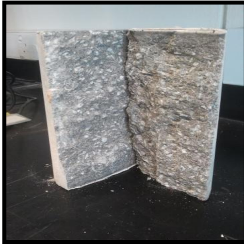
Figure 4.3 : Cube with no fiber addition
