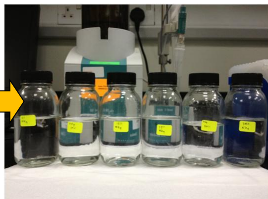
Figure 3.3: Aqueous (\text{NH}_4)_2\text{SO}_4 at 5, 8, 10, 12, 14, 15, 16 and 20 % w/v. 1ml of (\text{NH}_4)_2\text{SO}_4 at each concentration is added with 10ml bio-oil
