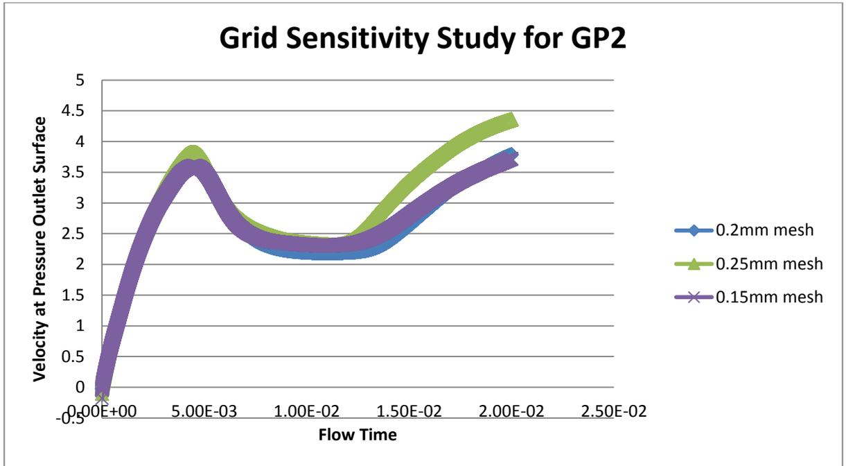
Figure 14: Graph of velocity against flow time for each of the grid sizes
