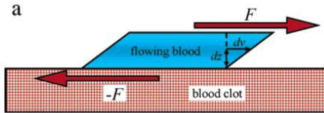
Figure 6: Viscous forces to dissolve blood clot when blood flow is laminar (Serza, Tratar, & Blinc, 2005)
