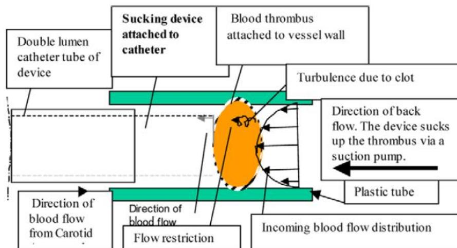
*Figure 1: 2D schematic view of GP device (Pearce, Patrick, & Perkinson, A New Device for the Treatment of Thromboembolic Strokes, 2007)*
