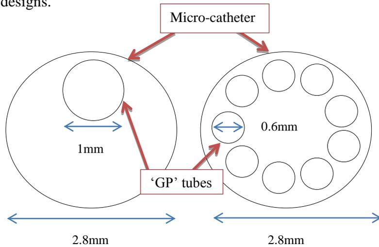
Figure 2: 2D sketch for the geometry of 'GP' device (left) and 'GP' 2 device (right)
