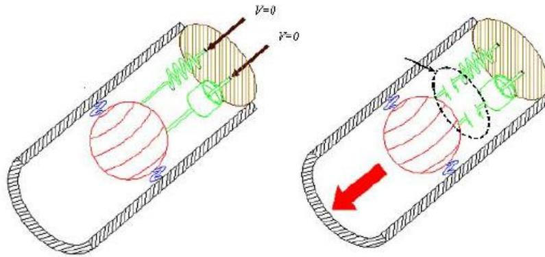
*Figure 5: Left figure shows the spring-damper system when force exerted is lower than the adhesion force; and the figure on the right shows when force exerted is equal or greater than the adhesion force (Romero, Higuera, Martinez, Pearce, & Perkinson, 2010)*
