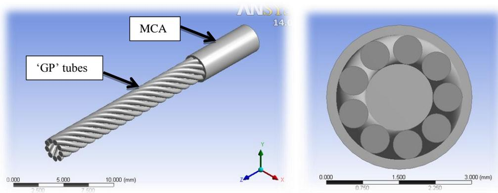
Figure 10: Isometric view (left) and front view (right) of 'GP' 2 device model 2
