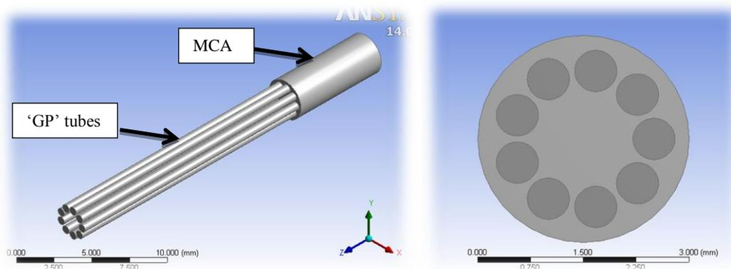
Figure 8: Isometric view (left) front view (right) of 'GP' 2 model 1
