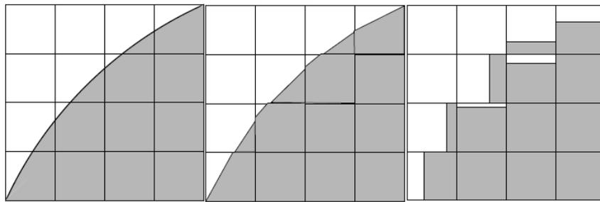
Figure 8: (a) Actual interpolation shape between phases; (b) interpolation by geometric reconstruction scheme; (c) interpolation by donor-acceptor scheme (Fluent 6.3 User Guide , 2006)
