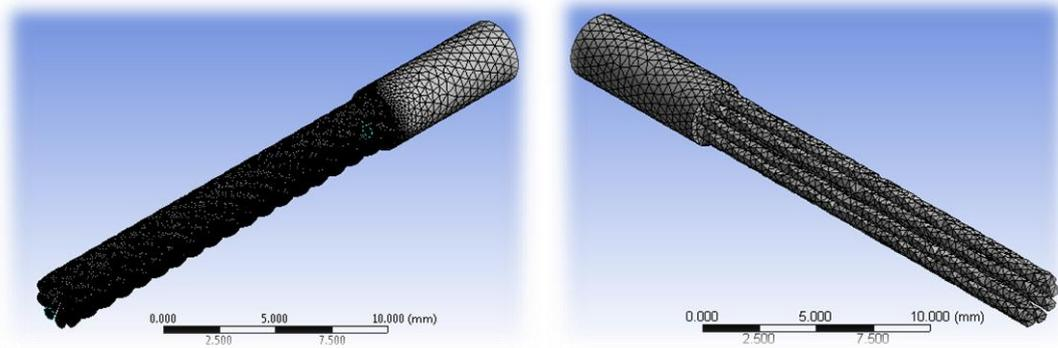
*Figure 12: Fine mesh (left) and coarse mesh (right)*
