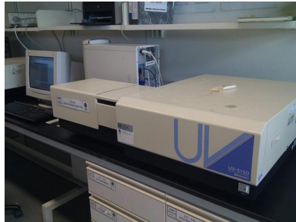
Figure 3.8: Apparatus and UV-VIS equipment to measure the optical density
