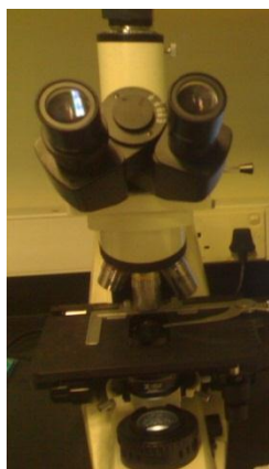
Figure 3.9: Microscope and counting chamber used to count the cell using Hemocytometer Method
