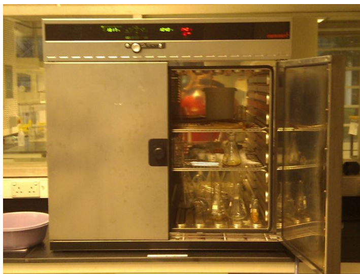
Figure 3.6: Oven used for drying process
