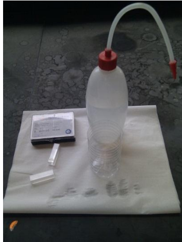
Figure 3.8: Apparatus and UV-VIS equipment to measure the optical density
