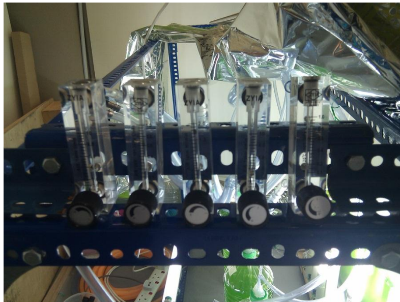
Figure 3.2: Flowmeter used to supply the air to photobioreactors
