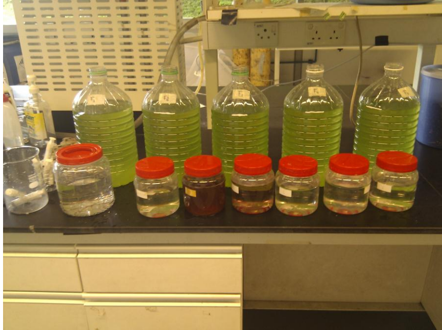
Figure 3.3: Limiting the nitrogen supplement to each photobioreactor
