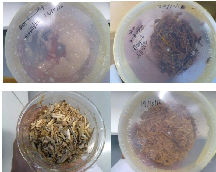
Figure 4.10 : Samples on microwave technique. (from left; glutinous rice, banana branch, thatch, palm oil frond)
