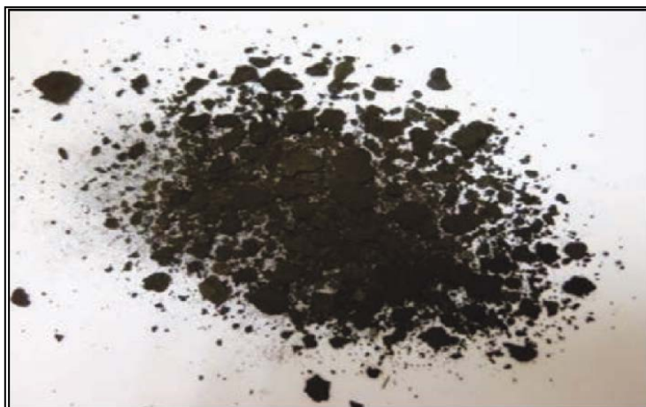
Figure 6: Deposits collected from reboiler tubes at Middle East Plant (Crew Energy Inc., 2011)
