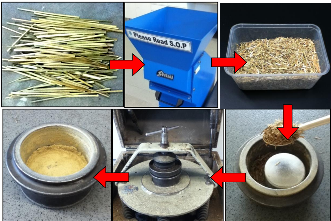
Figure 5: Process of machining the dried grass stem into particulate form for the fibre density measurement
