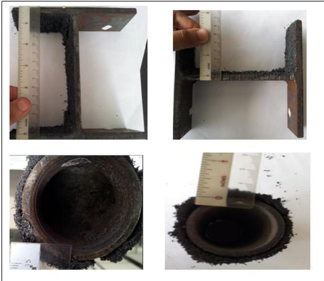
**Figure 7 : Char Expansion Measurement Method for I-Beam,
