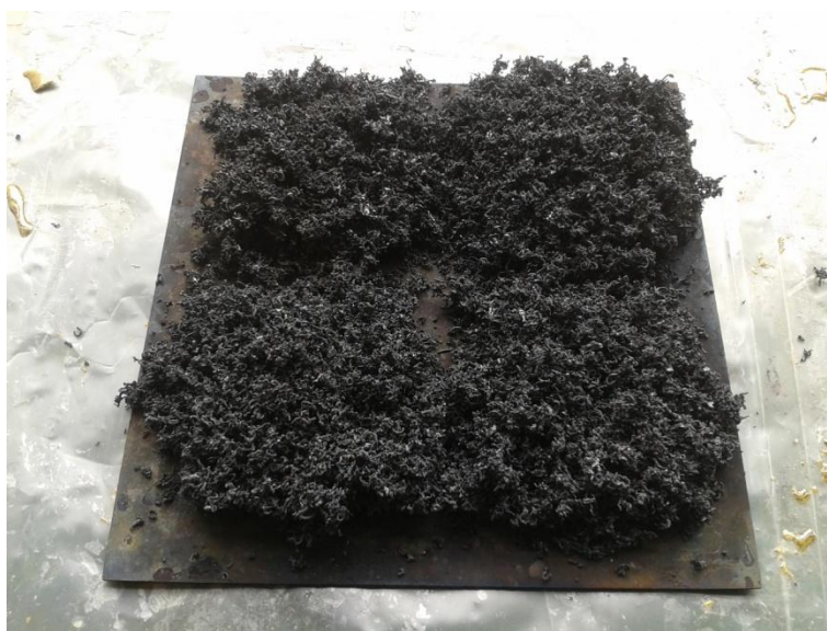
Figure 8: Residual char expansion
