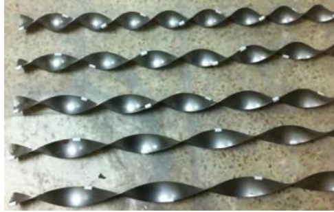
Figure 2.2: Coil plate inserts with different twist ratio (Halit et al., 2011)
