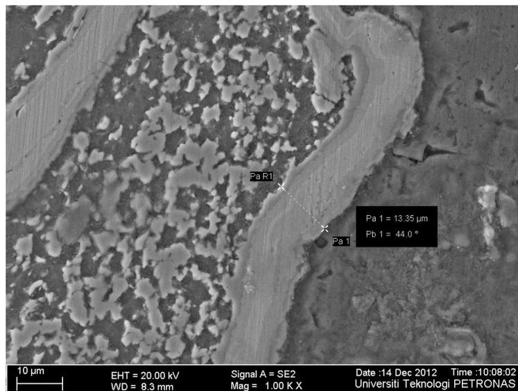
**Figure 25 : FESEM image that shows the thickness of Copper strip after FSP**
