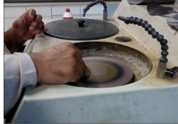
Figure 18 : Polishing process
