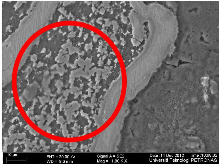
**Figure 24 : FESEM image of Nano MMC Al Cu (1000X magnification)**
