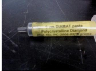
Figure 17 : Polishing solid paste
