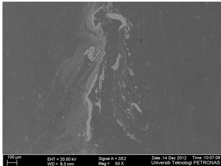
Figure 22 : FESEM image of Nano MMC Al Cu (50X magnification)
