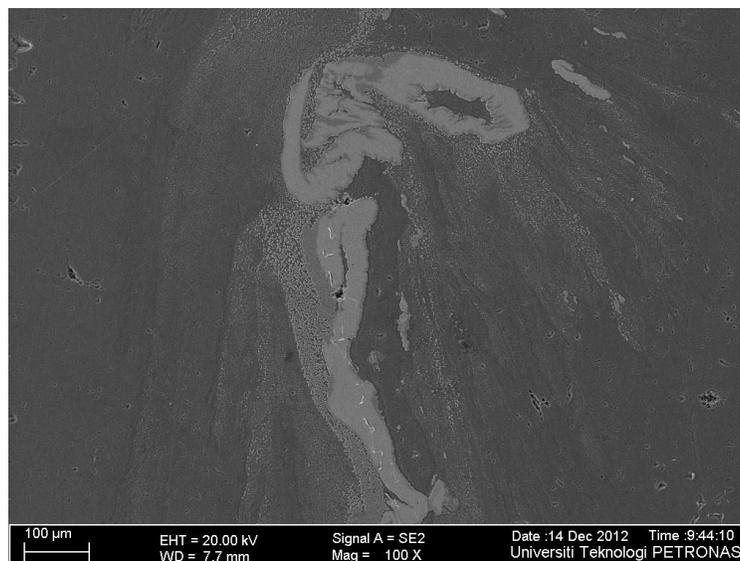
Figure 23 : FESEM image of Nano MMC Al Cu (100X magnification)
