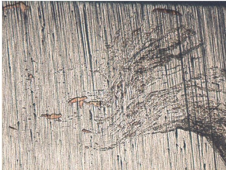
**Figure 20 : Microstructure image of MMC surface with 50X magnification**
