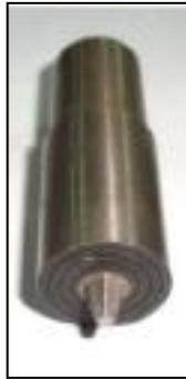
**Figure 6 : FSP tool (stainless steel)**
