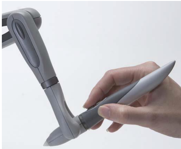
FIGURE 4.1.2.1.1 How to use PHANTOM Haptic Device
