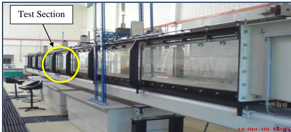
Figure 3.2: Water Flume / wave tank for the experiment
