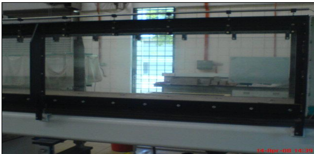
Figure 3.3: Test Section of the water wave flume
