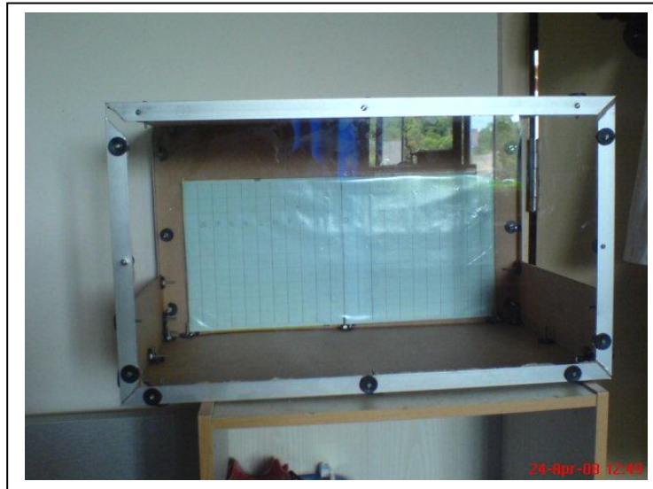
Figure 3.4: Test Section Box inserted into the water flume
