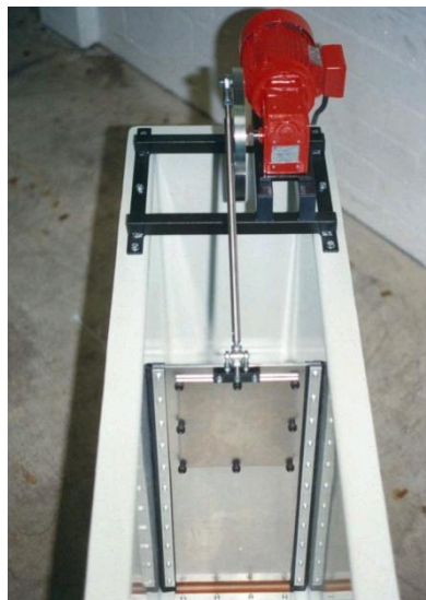
Figure 3.9: Motor and the flap to generate water waves
