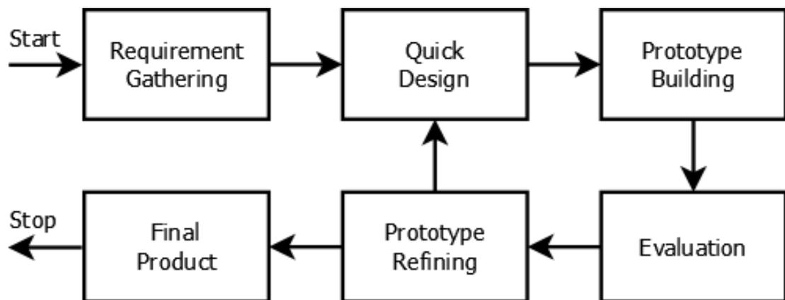
Figure 14 Prototyping development model
