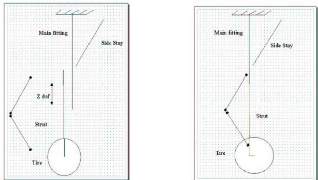
Figure 2-2: Proper landing gear model for the modal analysis [4]
