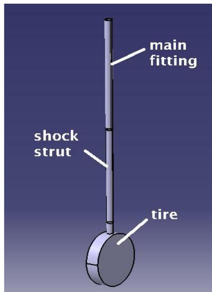
Figure 3-6: Modified model of the landing gear
