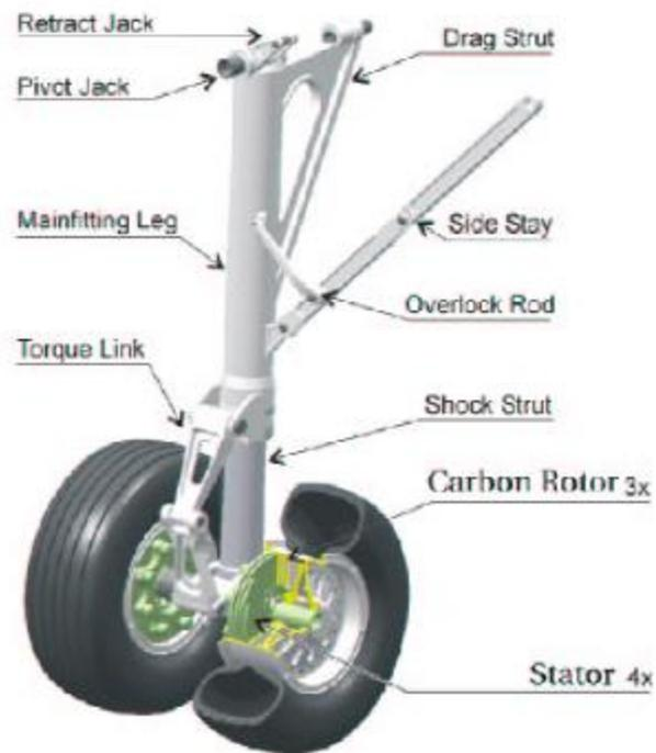
Figure 3-3: Landing gear model reference [7]
