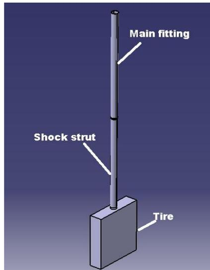
Figure 3-5: Simplified model with separated bodies
