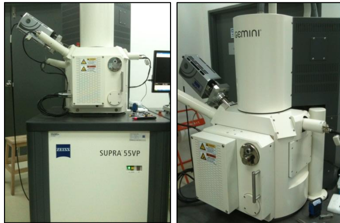
Figure 3.1: VP FESEM used for capturing samples' images [12]
