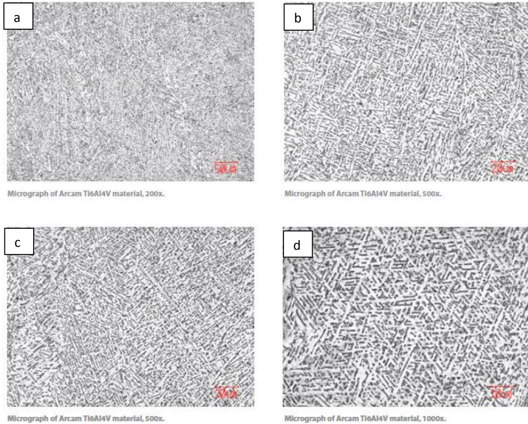
Figure 2.5: Micrograph of Arcam Ti6Al4V material: (a) 200X zoom, (b) 500X zoom, (c) 500X zoom and (d) 1000X zoom [7].
