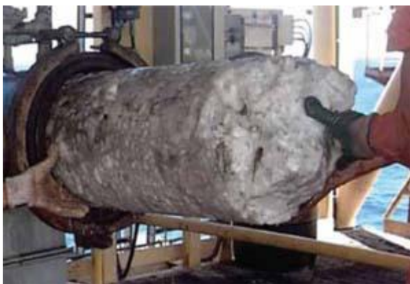
Figure 3: Formation of hydrates in pipeline [6].
