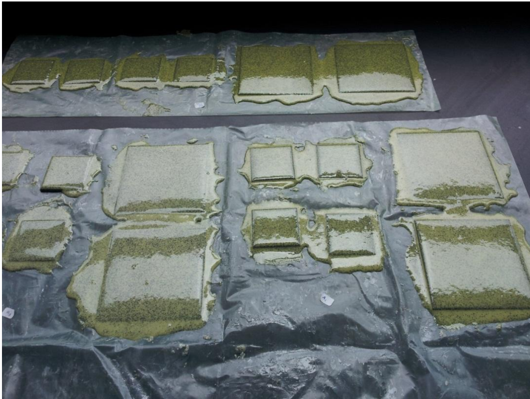
Figure 3-1: Coating curing on steel substrate
