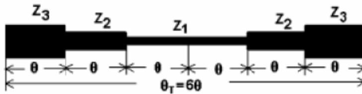
**Figure 7: Structure of the stepped impedance resonator**
