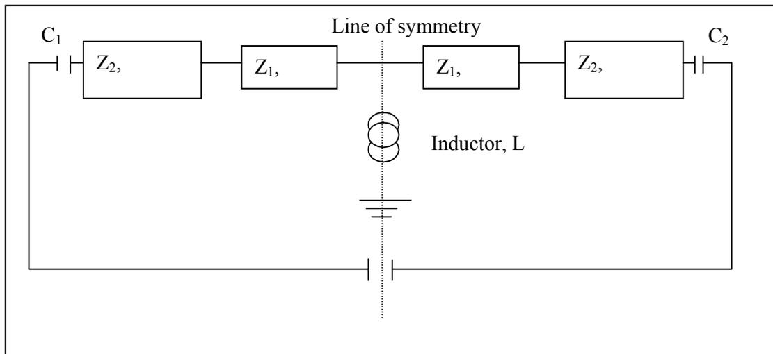
**Figure 11: Filter design topology**
