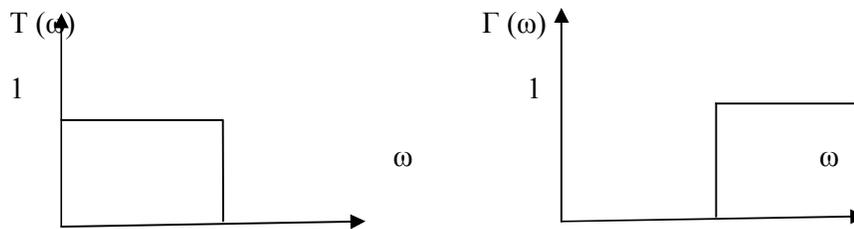
Adding to this, a linear phase response it would be a perfect microwave filter. There is one problem with these perfect filters, it is impossible to build. We must limit ourselves to filter functions which can only be expressed as finite polynomials.
