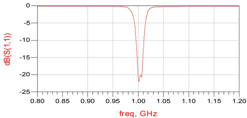
**Figure 18: Reflection Coefficient in Microstrip**
