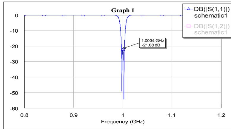
**Figure 15: Reflection coefficient response**
