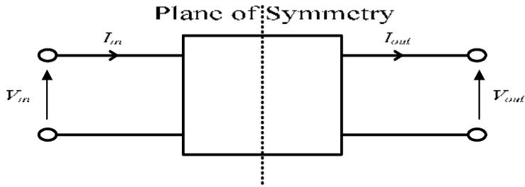
**Figure 2: Symmetrical two-port network**
