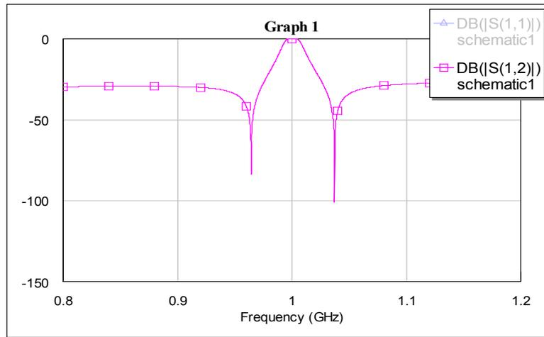
**Figure 14: Transmission coefficient response, S21**
