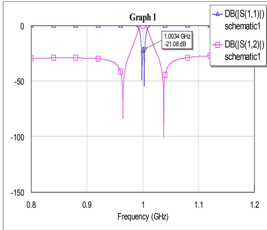
**Figure 13: Simulated quasi-elliptic filter response**
