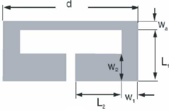
**Figure 9: Proposed folded stepped impedance resonator**
