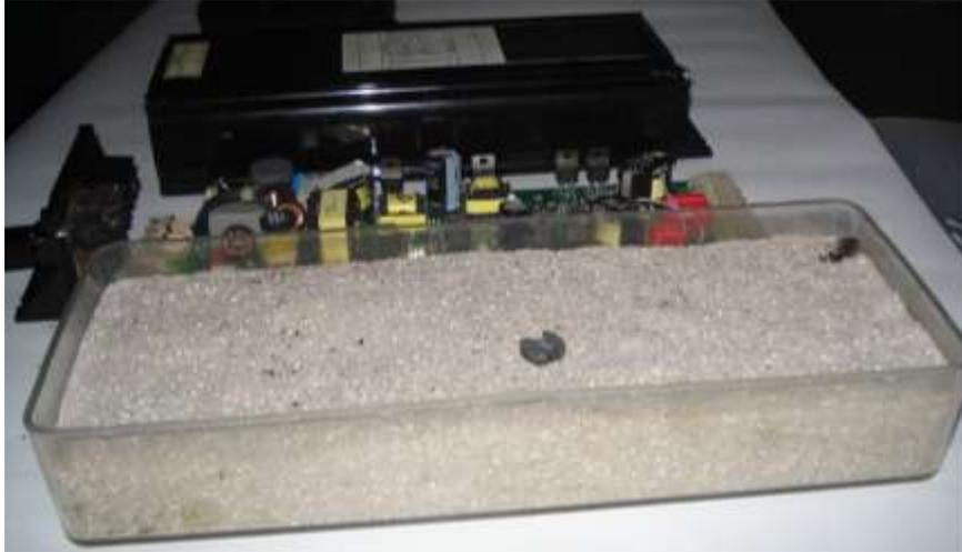
Figure 15: Sand inside the ballast casing
