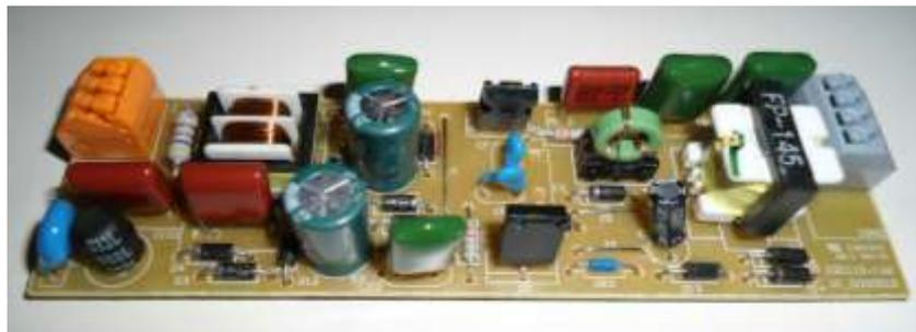
Figure 9 : Electronic ballast circuitry [13]
