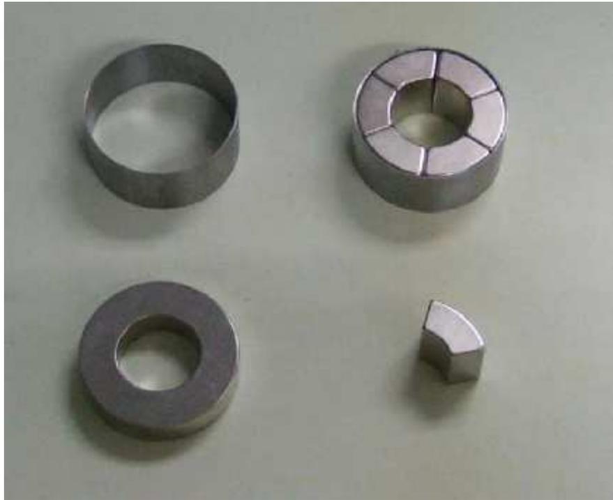
Figure 5.1 Ring and Segmented Magnet
