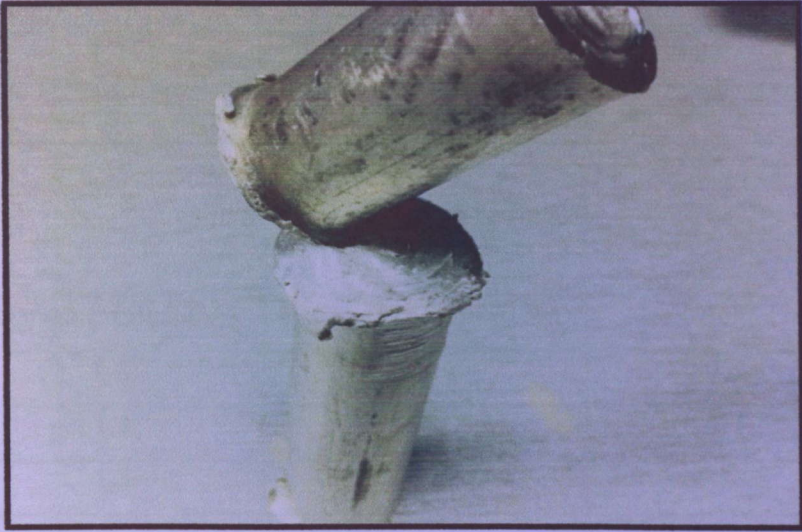
Figure 4.2.2.1 : Crooked Weld Joint (Side View)
