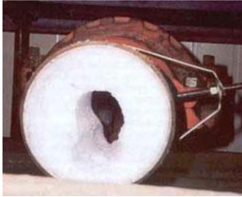
**Figure 1: Freeze formation inside pipeline (Products, 2012)**
