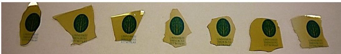
Figure 16: Comparison of the transparency of the mixed matrix membranes
