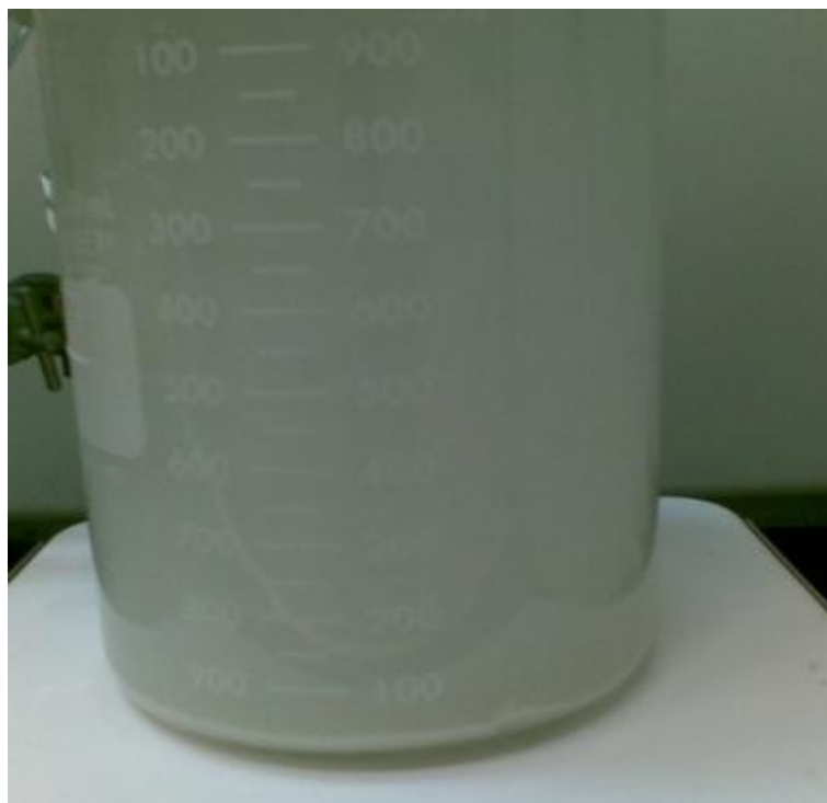
Figure 6: Low MW precipitate formed using 22.5wt% monomers in NMP solvent
