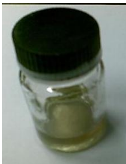
Figure 13: 7 wt% inorganic filler loading appears cloudy even after sonication
