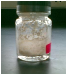
Figure 10: DCM cannot redissolve the polymer
