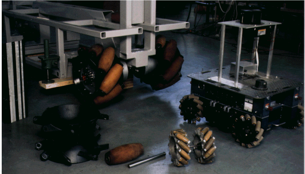
Figure 2.6: Robots using mecanum wheels at Robotic Institute, Carnegie Mellon University (CMU) [3].
