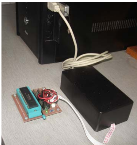
Figure 3.13: Microchips' In Circuit Debugger 2 (ICD2)
