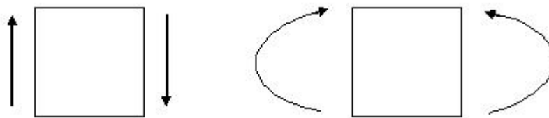
Figure 3.8: Normal positive shear force convention (left) and normal bending moment convention (right).
