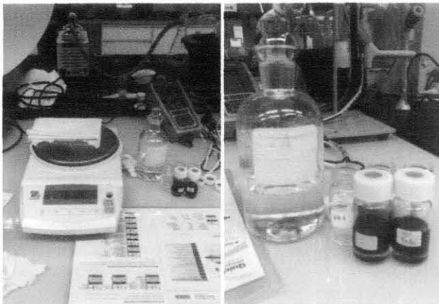
Figure 5: 5 grams of UEO and 5 grams of IL (HEF) are carefully measured and placed in a bottle, which are then sent for centrifuging at 500 rpm for 30 mintues.
