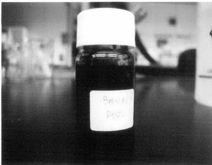
Figure 17: BmimAc + Diesel + Water after 3 days being left for separation.
