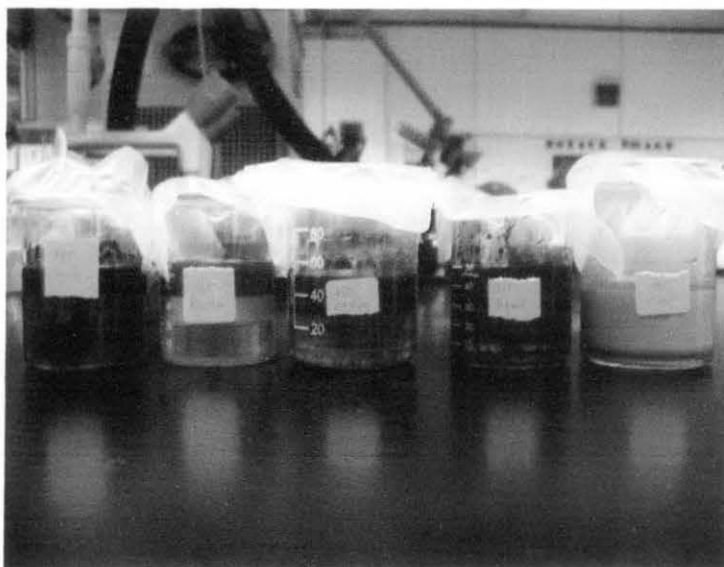
Figure 10: UEO + HEF stirred with water after 3 days being left for separation. From the left is Toyota, Perodua, Random, Diesel, Motor.
