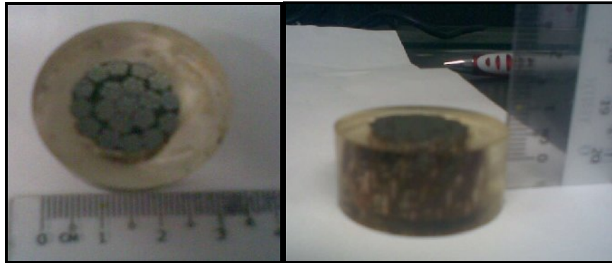
Figure 3.8: Mounted specimen using cold mounting
