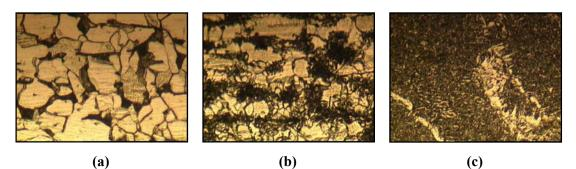
Figure 4.2: Microstructure of weld region under 20X magnification of (a) Base Metal, (b) HAZ, and (c) Weld Metal
