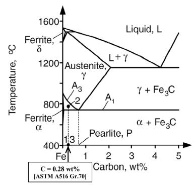
Figure 4.6: Mechanism of partial grain refining in carbon steel [11]
