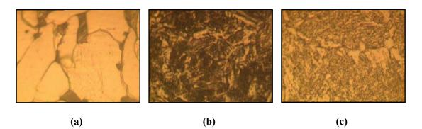
Figure 4.3: Microstructure of weld region under 50X magnification of (a) Base Metal, (b) HAZ, and (c) Weld Metal
