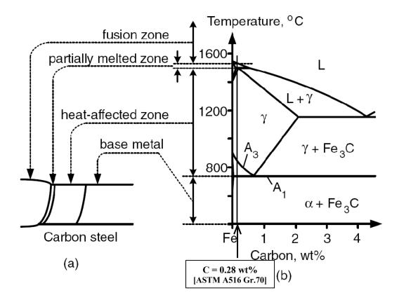
Figure 4.5: Carbon steel weld: (a) HAZ; (b) phase diagram [11]
