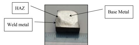
Figure 4.1: Macrography of the welded section.
