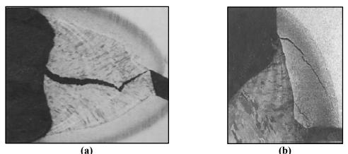
Figure 2.2: Example of Cracking at (a) Weld Metal, and (b) HAZ
