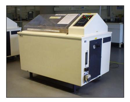
Figure 3.2: Cyclic Corrosion Cabinet Model SF/450/CCT
