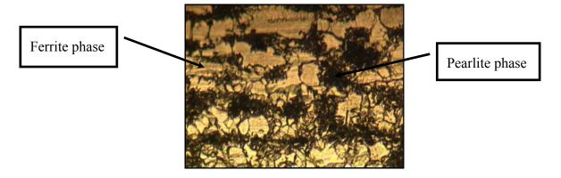
Figure 4.8: Microstructure of Pearlite and Ferrite after grain refining process
