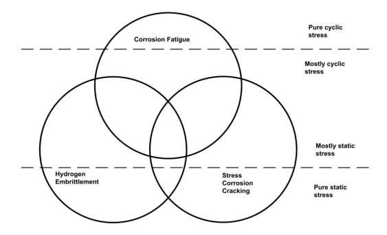
Figure 2.1: Venn diagram illustrating the interrelationship between stress corrosion cracking, corrosion fatigue, and hydrogen embrittlement [3]
