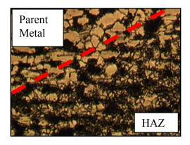
Figure 4.4: Microstructure of HAZ and PM with 10X magnification.
