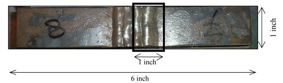
Figure 3.3: Size (1 inch<sup>2</sup>) of section cut from original specimen
