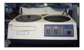
Figure 3.5: Grinding machine
