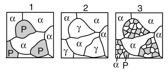
Figure 4.7: Pearlite (P) colonies transform to austenite ( $\gamma$ ) and expand slightly into the prior ferrite ( $\alpha$ ) colonies upon heating to above A<sub>1</sub> and then decompose into extremely fine grains of pearlite and ferrite during cooling [11].
