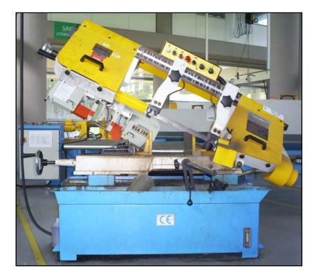
Figure 3.4: Bend Saw Machine
