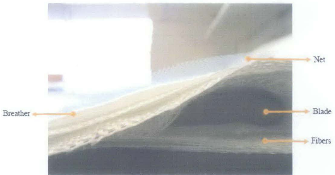
Figure 3.2: Arrangement of blade, fibre, net and breather.
