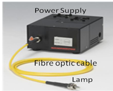
Figure 3.3: High power Tungsten-Halogen Light Source (Hamamatsu, 2009).
