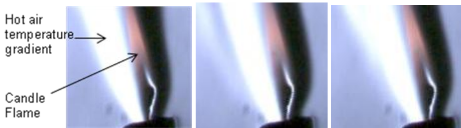
Figure 4.34: Several images of schlieren by using UTP Automotive Center schlieren system.
