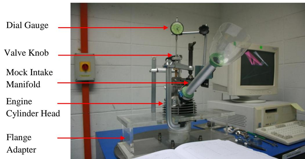
Figure 4.2: Engine cylinder head and mock intake manifold setup
