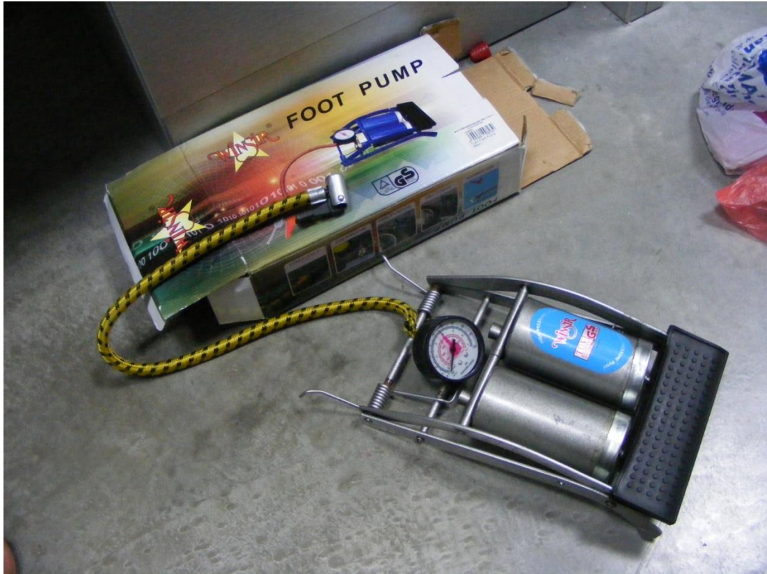
Fig 4.6: Foot pump sourced for piston-cylinder assembly
