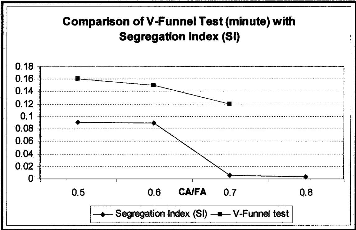
Figure 19: Comparison of result between V-Funnel Test and Segregation Index (SI)
