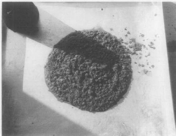
Figure 8: Slump flow without segregation
