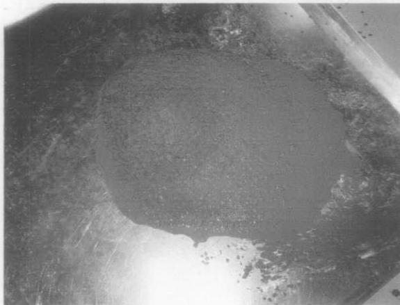
Figure 9: Slump flow with segregation
