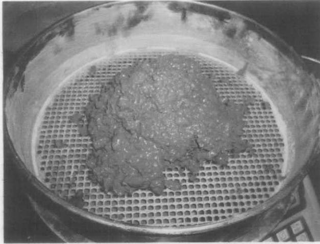
Concrete was poured onto the 5mm mesh
