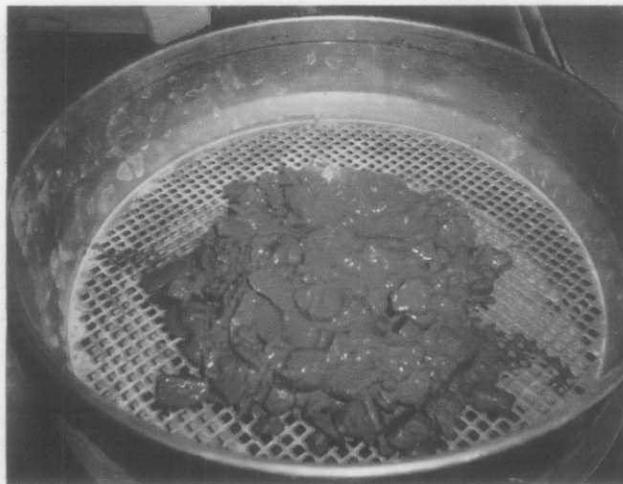
Concrete was poured onto the 5mm mesh
