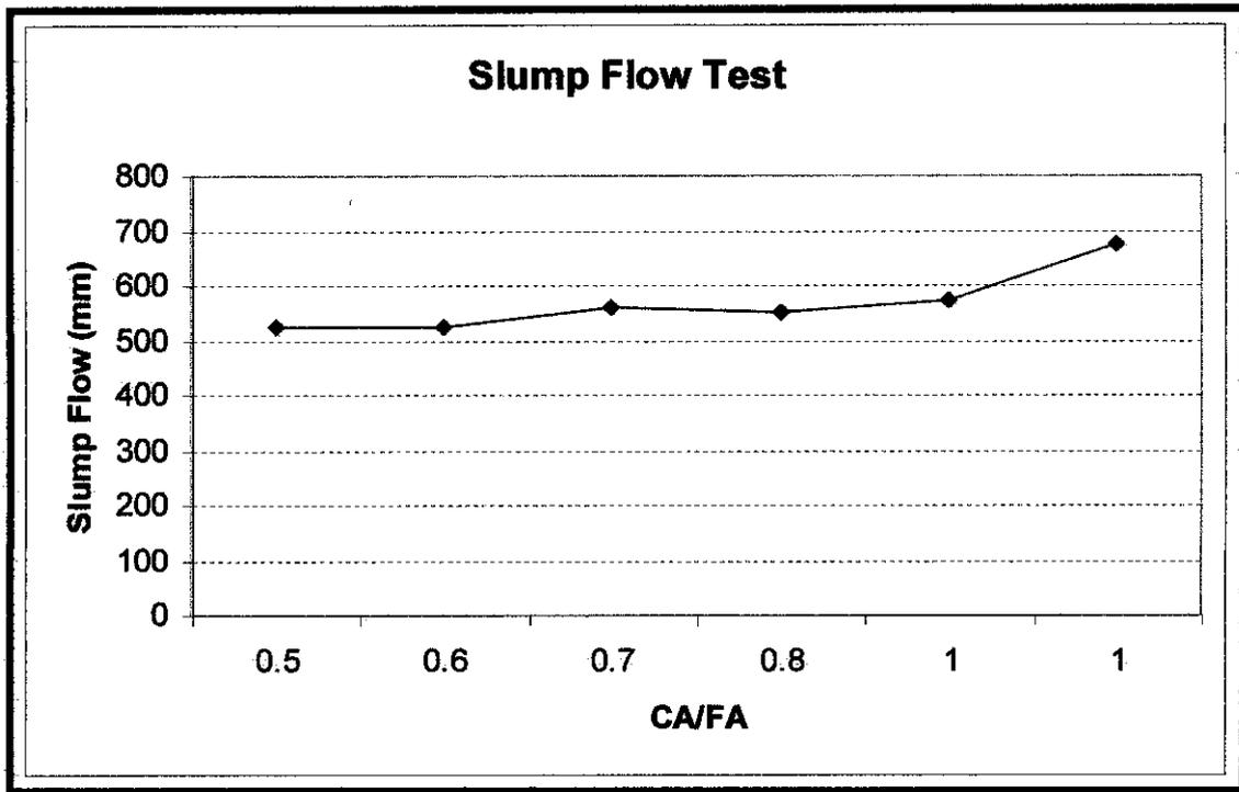
Figure 13: Slump Flow Test Evaluation
