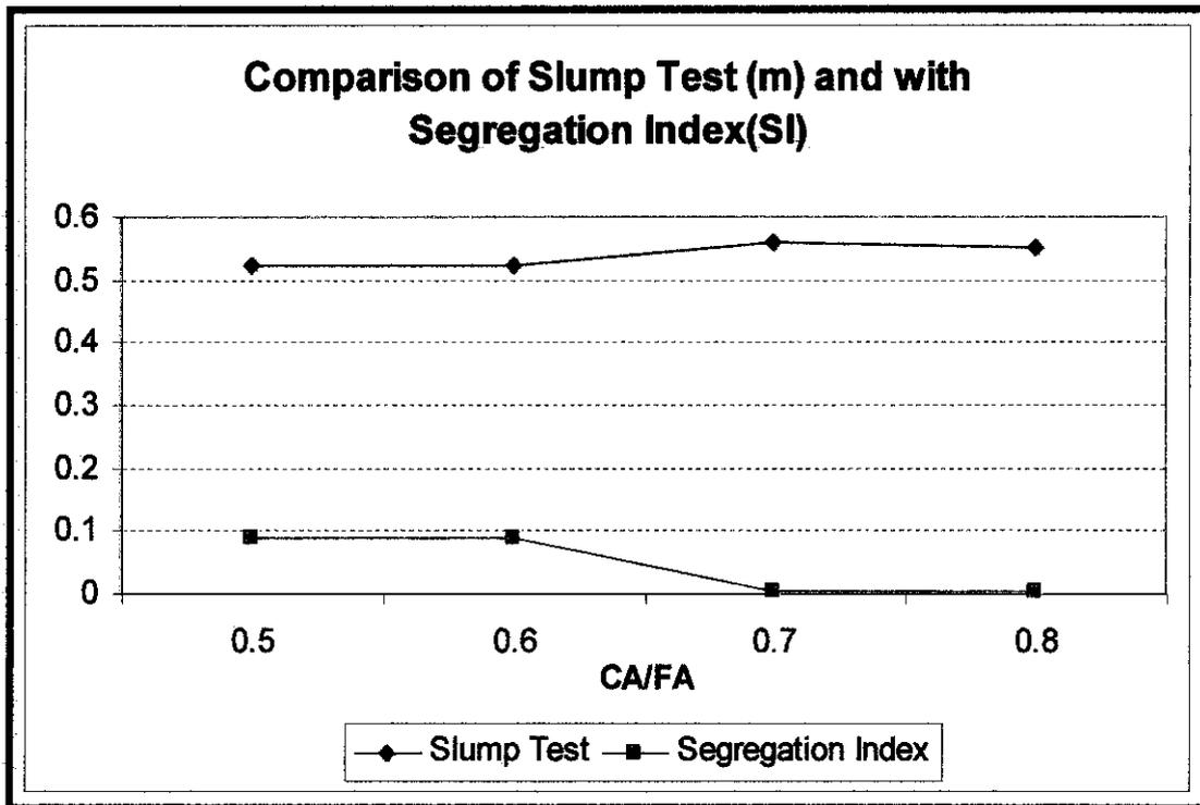
Figure 18: Comparison of result between Slump Test and Segregation Index (SI)
