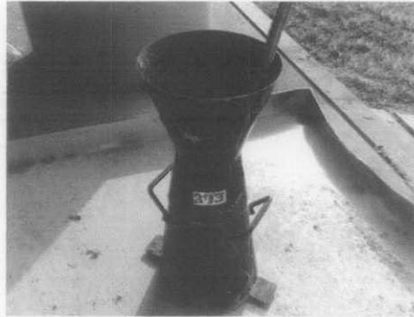
The truncated cone for slump flow test
