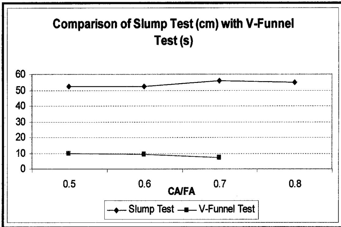
Figure 17: Comparison of result between Slump Test and V-Funnel Test
