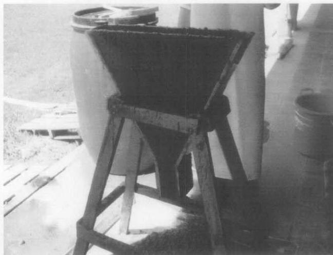
Concrete was falling free out of the funnel
