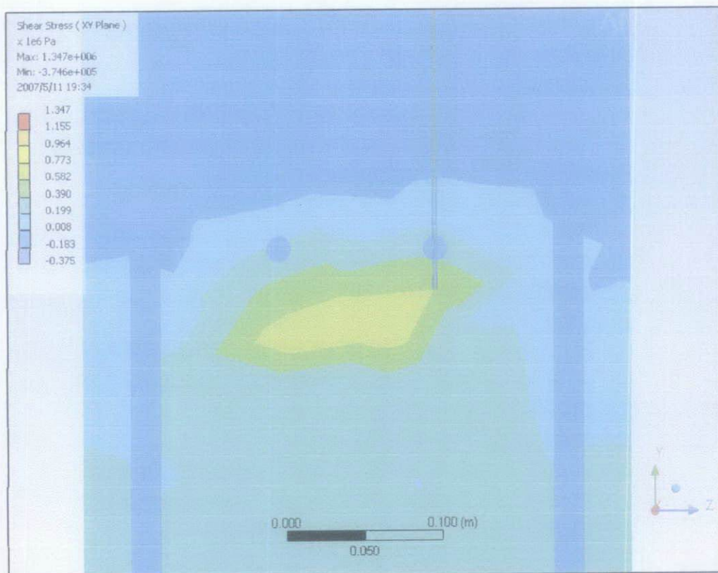
Figure 4.16b: Bond Stress (beam)
