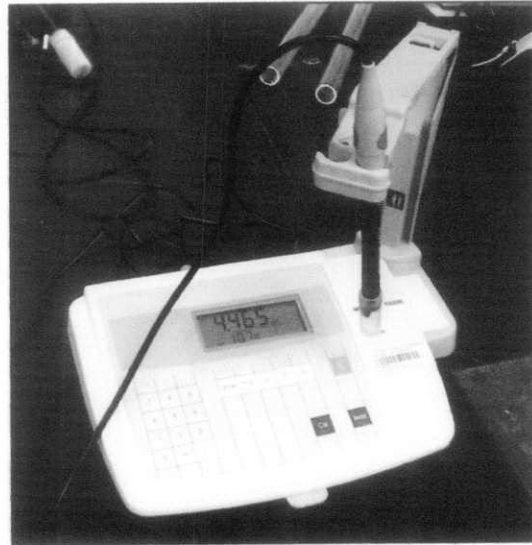
Figure 3.14: Mettler Toledo model MP230 pH meter
